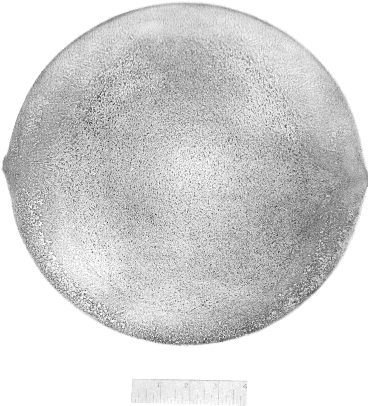
Figure 7. Typical Macro-Etched Section from the Middle of the Forging
