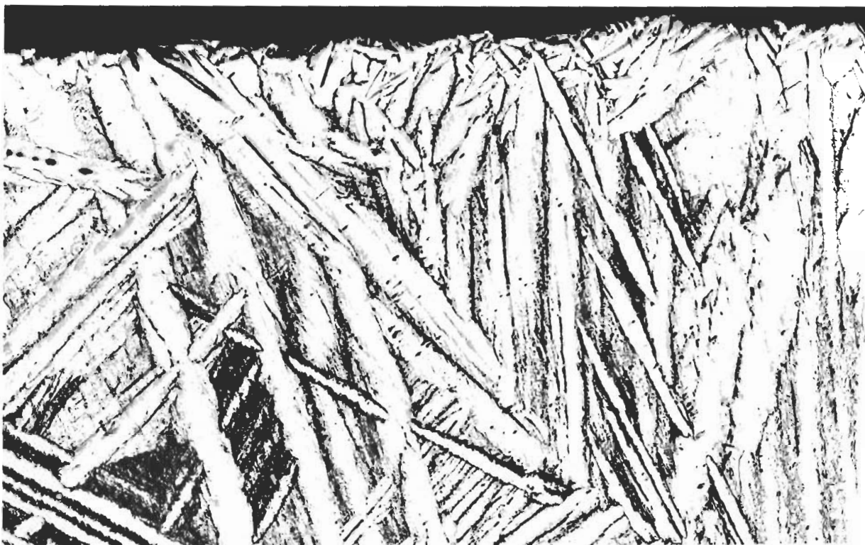
Figure 56 - Surface of Casting from Zircon Shell Mold Sectioned through 3/4 inch Diameter Base Modified Kroll's Etch 75X
