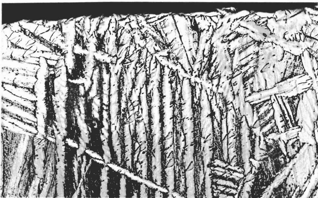
Figure 57 - Surface of Casting from Zircon Shell Mold Sectioned through 2 inch Diameter Top Modified Kroll's Etch 75X
