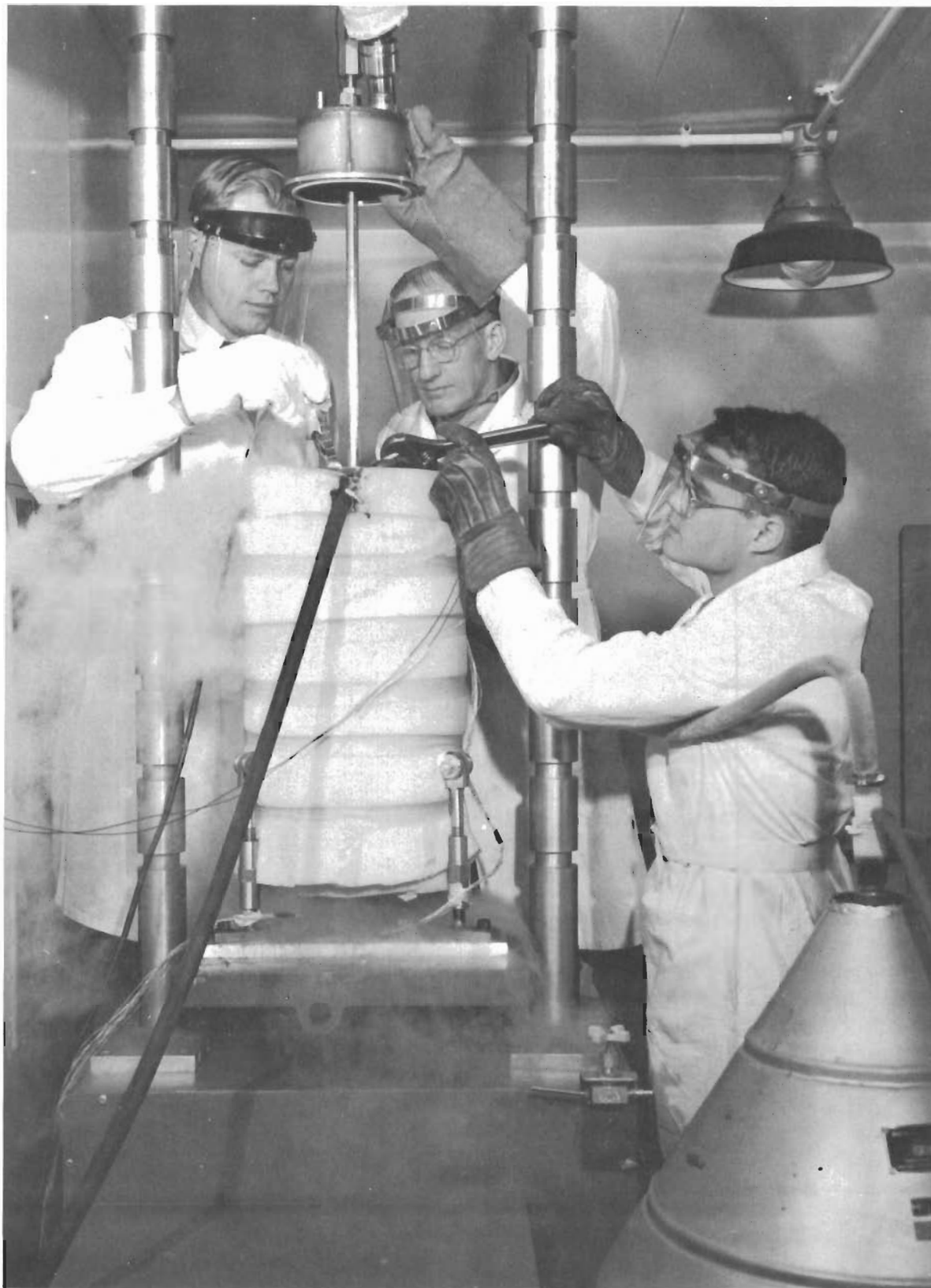
Figure 18. Liquid-Hydrogen Test Chamber Being Prepared for Test
