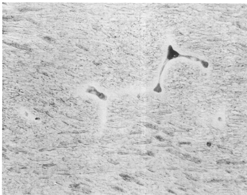
FIGURE 7. MICROSTRUCTURE OF HIGH-PHOSPHORUS SAE 4340-TYPE STEEL SHOWING UNKNOWN PHASE (DARK) WITH HIGH-ALLOY AREA (LIGHT)
