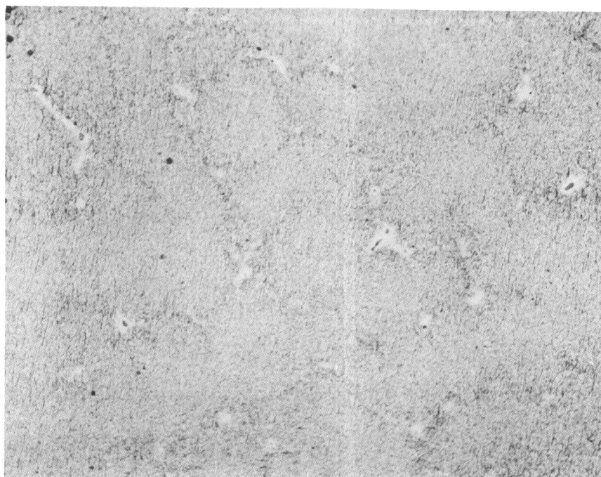
FIGURE 6. MICROSTRUCTURE OF HIGH-PHOSPHORUS SAE 4340-TYPE STEEL
