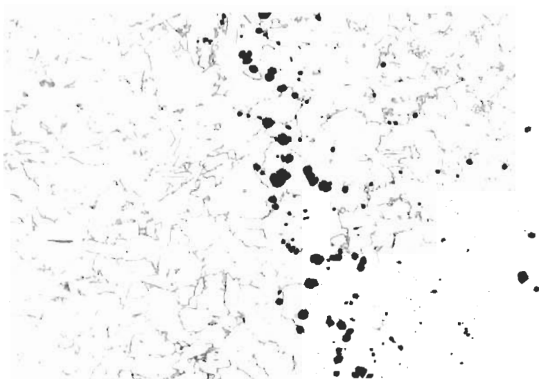
Figure 8. An Example of Moderate Graphitization at the Low-Temperature Edge of a Weld-Heat-Affected Zone
