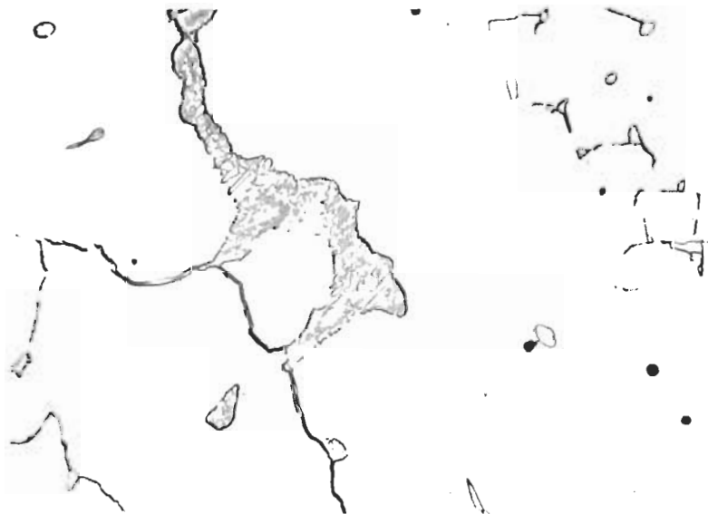
Figure 4. A 20 Cr-9 Ni Alloy as Cast. Eutectic Carbides, Some Intergranular Carbides and Occasional Islands of Delta Ferrite are Present
