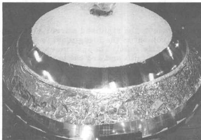
Figure 21 - Mirror with Double- and Single- Thickness Predistributed Foam
