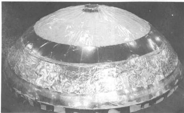
Figure 22 - Mirror with Back Flap
