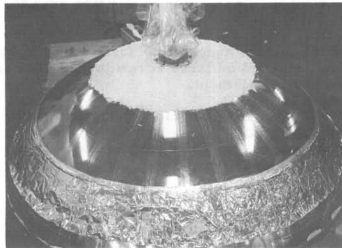
Figure 20 - Predistributed Foam Applied to One-Half of Mirror Area
