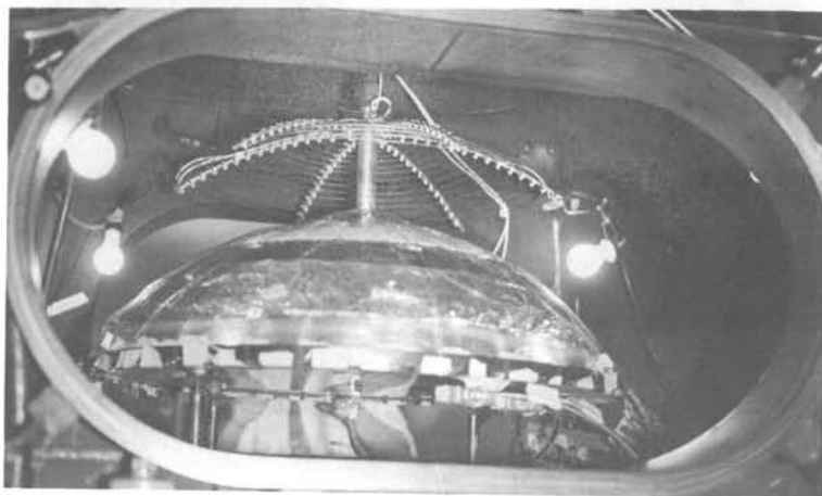
Figure 23 - Mirror in Vacuum Chamber
