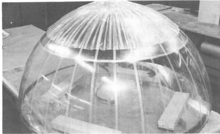
Figure 19 - Hemispherical Assembly of Inflated Solar Concentrator
