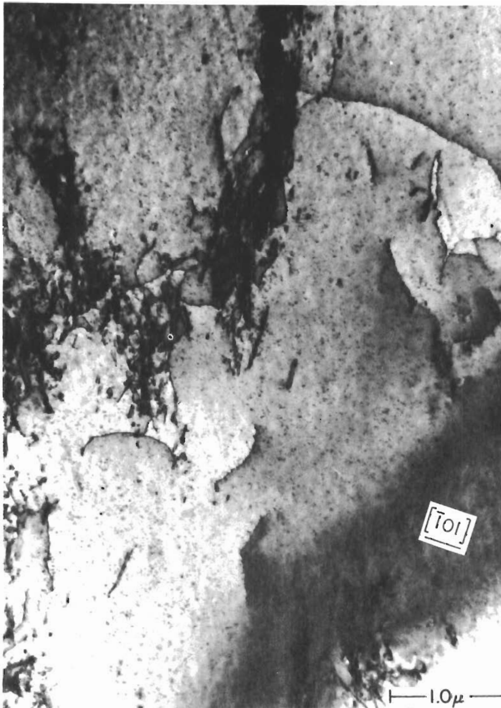
Figure 18 - Copper Single Crystal M6 (Irradiated); N = 20. Isolated dislocations in an irradiated specimen.
