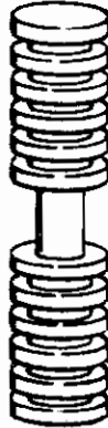
b. Grooves and gage length machined on spark-cutting machine using a lathe attachment
