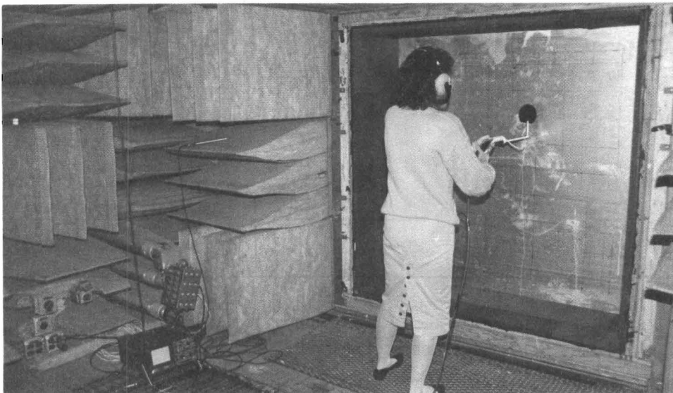
Figure 6. Intensity Probe Survey of the Test Panel Inside the Anechoic Room
