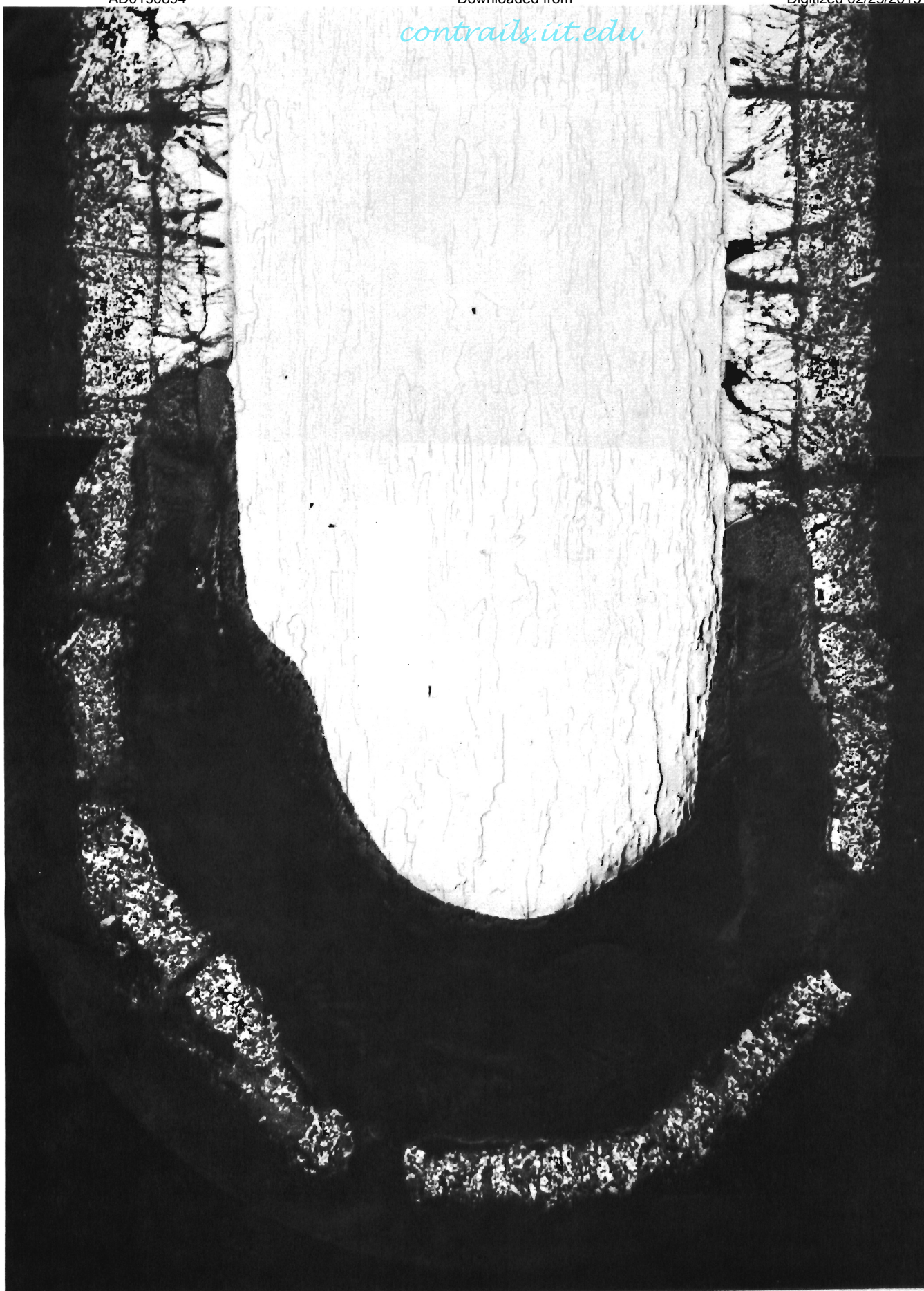
FIGURE 41 (M5266, M5267) Polish-Etch-Buffer SPECIMEN D289. MICROSTRUCTURE OF CROSS SECTION AT FAILED EDGE OF TEST PANEL, SHOWING PROGRESS OF OXIDATION.
