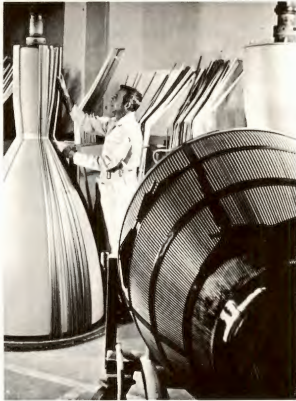
FIGURE 8. CONSTRUCTION OF COMBUSTION CHAMBER
