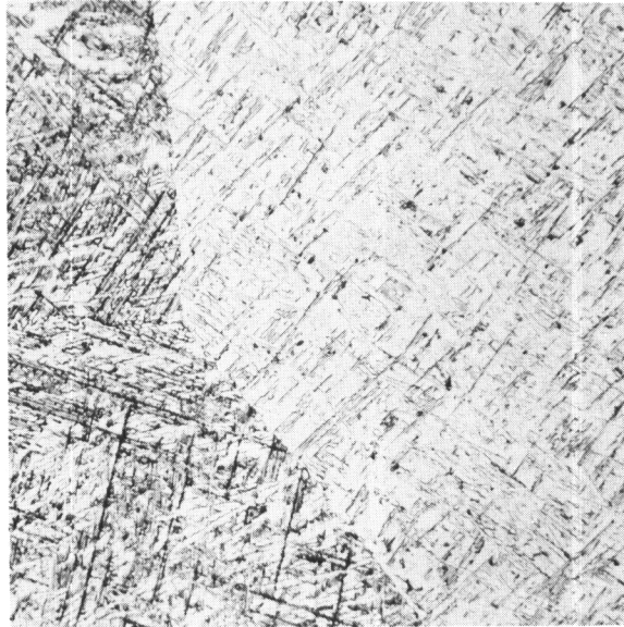
FIGURE 22. 2.91 PER CENT MANGANESE ALLOY ISO-THERMALLY TRANSFORMED FOR 312 HOURS AT 550 C
