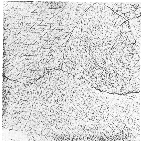
FIGURE 10. HEAT WT42A, A Ti-3.5Cr-3.5V ALLOY ROLLED AT 1600 F, HEAT TREATED AT 1300 F, AND WATER QUENCHED
