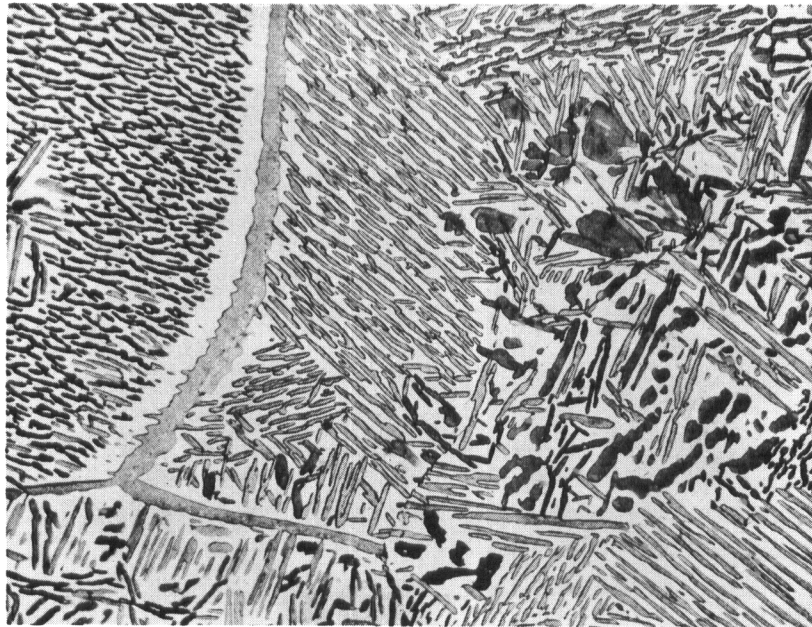
FIGURE 69. Ti-7.54Cr ALLOY ISOTHERMALLY TRANSFORMED FOR 72 HOURS AT 1202 F (650 C)
