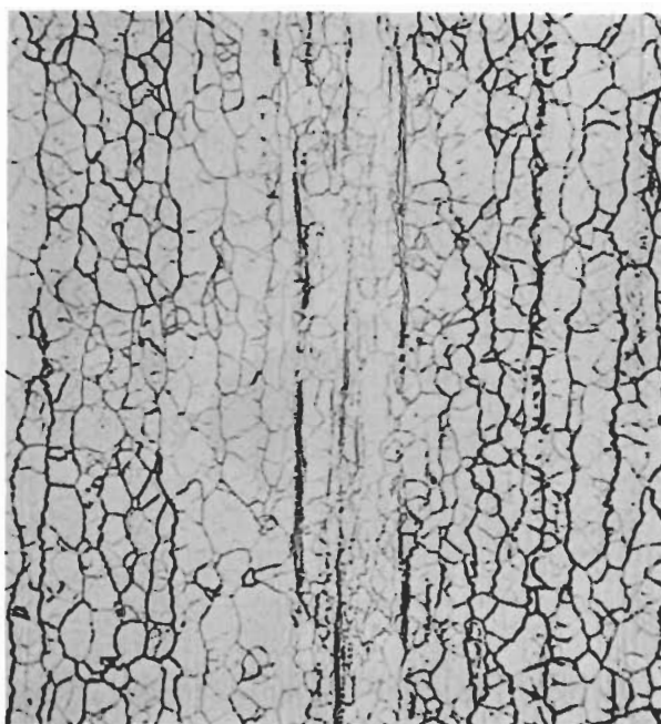
Figure 81 Flash Weld in D31, Weld No. 26
