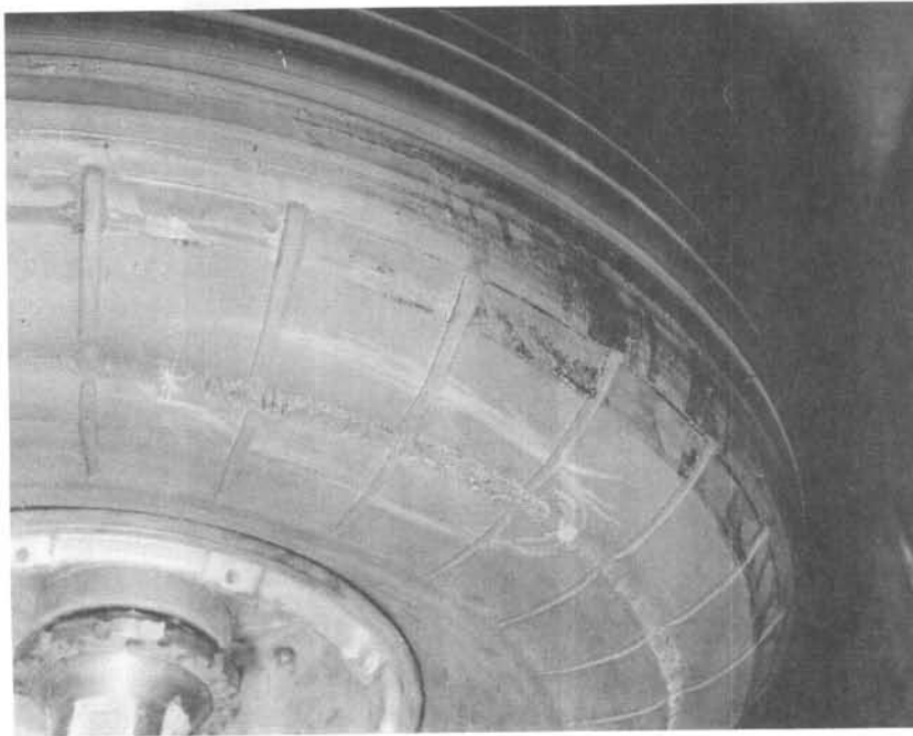
a) Continuous Flow Cracks
