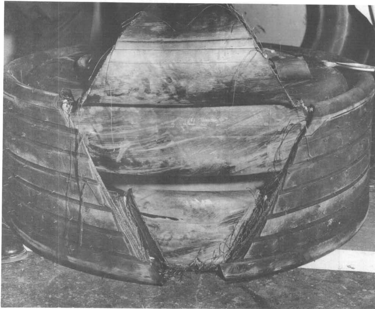
FIGURE 31. 23.00-20 Expandable Tire, Number L-1, After Hydrostatic Burst
