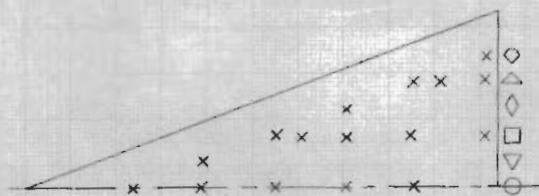
Fig. 32 - Chordwise Pressure Distribution on Flat 70° Delta Wing at M_{\text{apex}}=12.6 , Re/ft = 2.13 \times 10^5
