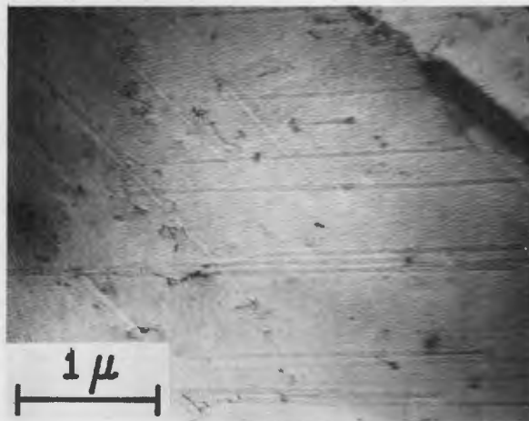
FIG. 16 -- TRAILS OF MOVING DISLOCATIONS IN IRON B-3.
