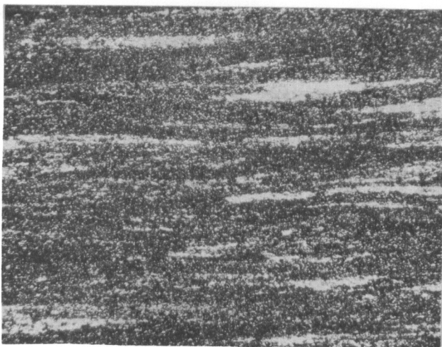
Figure 11. Commercial Ti-3% Mn sheet, longitudinal edge that exhibited shear cracks. Structure thought to be beta stringers (light) in equiaxed alpha-beta matrix (dark).
