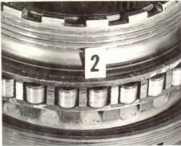
FIGURE 12. NO. 2 BEARING ROLLERS, CAGE AND INNER RACE
