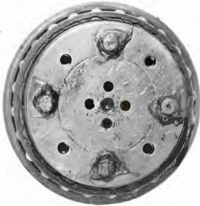
FIGURE 4. ERDCO TEST BEARING AFTER 100 HOURS OF RUNNING
