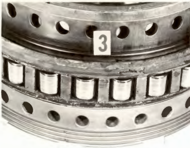
FIGURE 16. NO. 3 BEARING ROLLERS, CAGE AND INNER RACE
