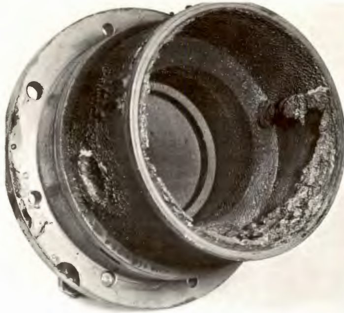
FIGURE 7. BEARING CHAMBER DEPOSITS
