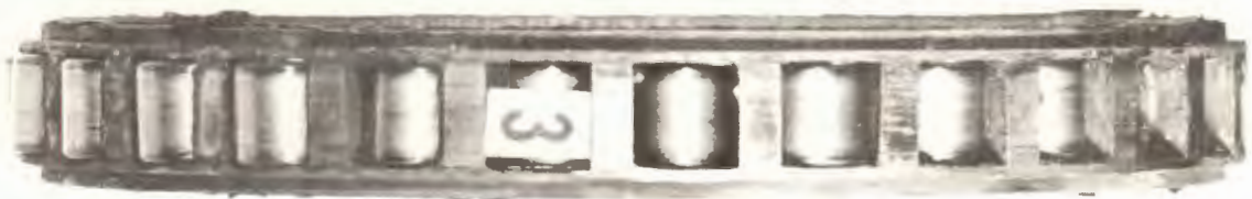
FIGURE 19. NO. 3 BEARING ROLLERS AND CAGE
