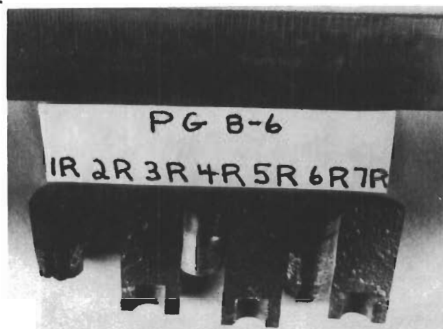
Figure 123. Post Exposure Photographs of Arc Plasma Tests PG(B-6)-1R, 2R, 3R, 4R, 5R, 6R and 7R, "C" Axis Perpendicular to Arc. Hot Face Pointing Up. One Inch Scale. Samples 3R, 5R and 7R Show "C" Plane Delaminations. Sample PG(B-6)-5R Delaminated on "C" Plane During Installation Due to Interference Between Stinghole and Sting.
