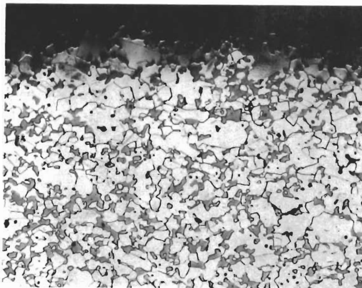
Figure 71. Arc Plasma Test \text{HfB}_{2.1} + 20 \text{ v/o SiC(A-7)-28R} Average Surface Temperature 4650^\circ \text{F} , Exposure Time 22, 400 Seconds (13 cyclic exposures each of approximately 1800 seconds), Stagnation Pressure 0.07 Atm. Stagnation Enthalpy 10300 BTU/lb, Cold Wall Heat Flux 495 BTU/ft 2 sec, 15 Mils Recession, Hot Face Up. One Inch Scale.
