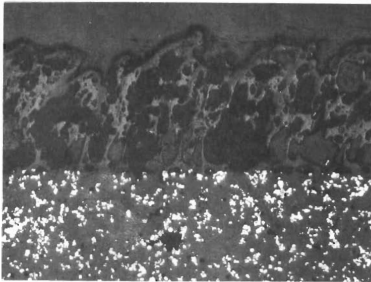
Figure 272. Arc Plasma Test \text{SiO}_2 + 60\text{w/oW(H-23)-8R} . Hot Interface Showing Some \text{SiO}_2 Reaction.
