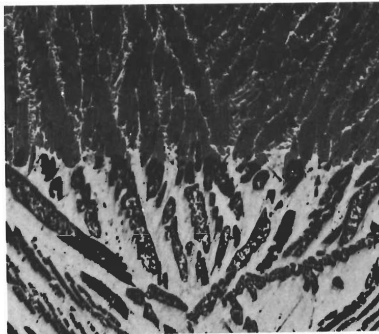
Figure 290. Arc Plasma Test Hf-Ta-Mo(I-23)-38MH Surface Temperature 4230 o F, Exposure Time 1800 Seconds, Stagnation Pressure 1.02 Atm., Stagnation Enthalpy 3220 BTU/lb, Cold Wall Heat Flux 435 BTU/ft 2 sec, 48 Mils Recession, Hot Face Up. One Inch Scale
