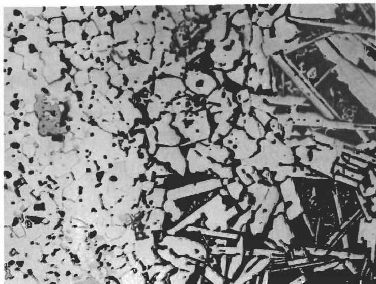
Figure 23. Arc Plasma Test HfB 2.1 (A-2)-10R. Rapid Melting was Observed. Interface of Melted Region (Right) and Matrix.
