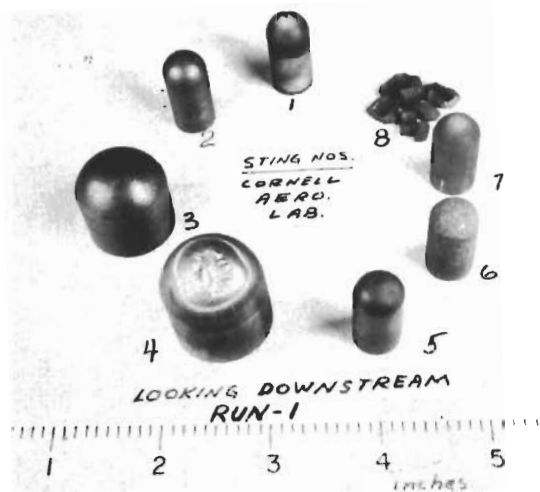
Figure 334. CAL Run 67-473, Mach Number 5.45, Stagnation Pressure 1.15 atm, Stagnation Enthalpy 2200 BTU/lb, Cold Wall Heat Flux 580 BTU/ft 2 sec, Exposure Time 15 Seconds.
