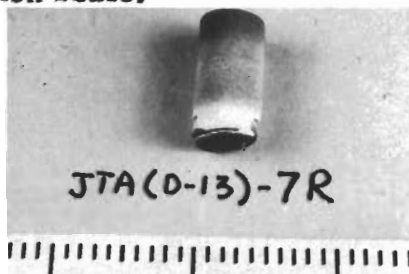
Figure 182. Post Exposure Photographs of Arc Plasma Tests JTA(D-13)-8R and 9R (Hot Face Up) and 7R (Hot Face Down). One Inch Scale.
