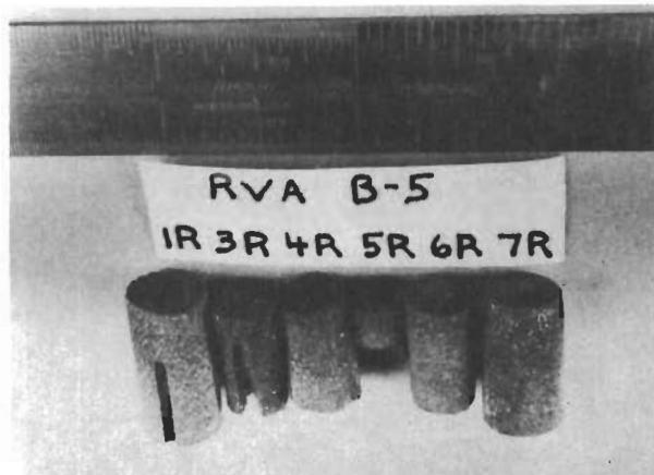
Figure 116. Post Exposure Photographs of Arc Plasma Tests RVA (B-5)-1R, 3R, 4R, 5R and 7R. Hot Face is Pointing Up. Samples 1R and 3R Show Exposed Thermocouple Holes While 5R Shows Sting Hole Exposed Due to Side Ablation.
