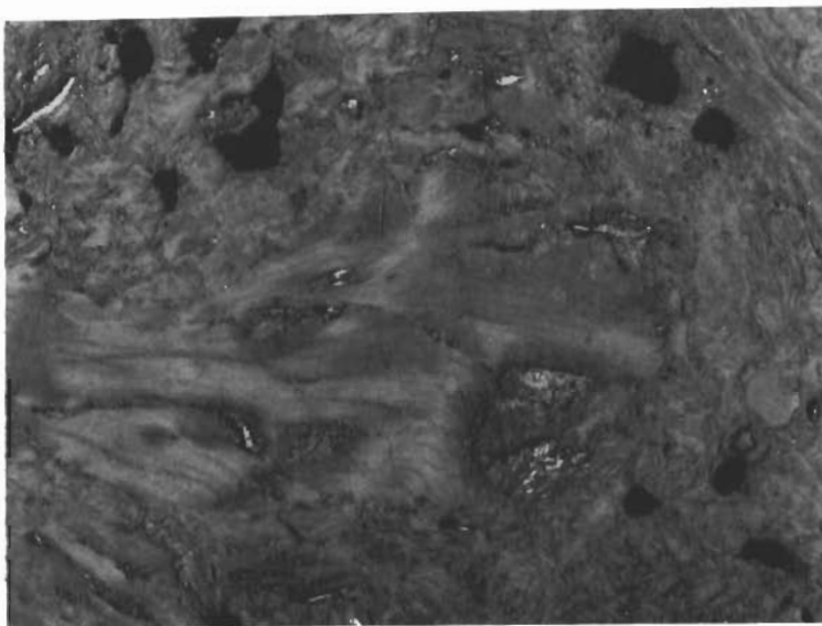
Figure 121. Arc Plasma Test RVA(B-5)-7R, Matrix Area. Little Difference Noted between Interface and Matrix.
