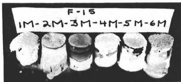
Figure 206. Post Exposure Photographs of Arc Plasma Tests JT0992 (C-HfC-SiC) (F-15)-1M, 2M, 3M, 4M, 5M and 6M. Hot Face Pointed Up.
