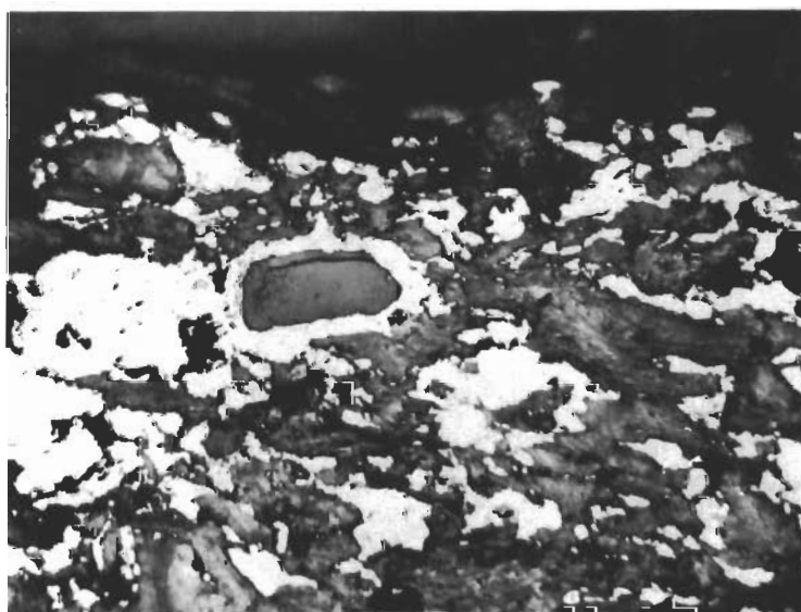
Figure 191. Arc Plasma Test JTA(D-13)-7R. Oxide Detached at Top Interface.
