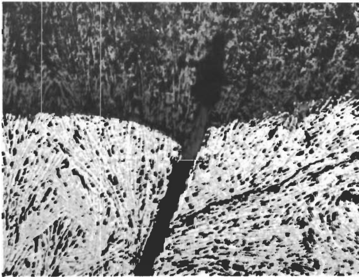
Figure 179. ZrC+C(C-12)-5M. Interface of Oxide (Top) and Carbide Matrix.
