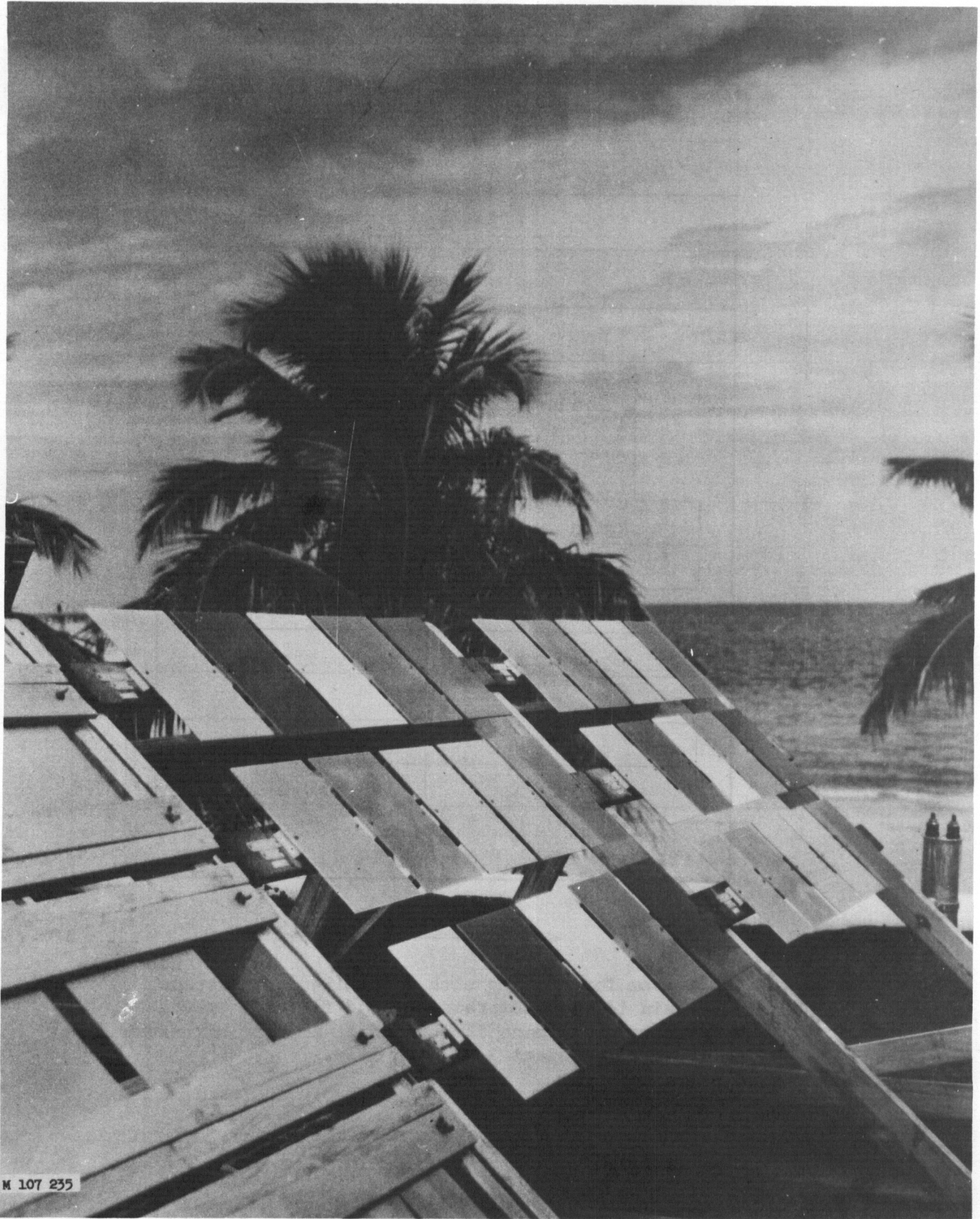
Figure 6--Method of mounting subpanels on boards and exposure racks. Photograph shown is of the salt air exposure site in Florida.
