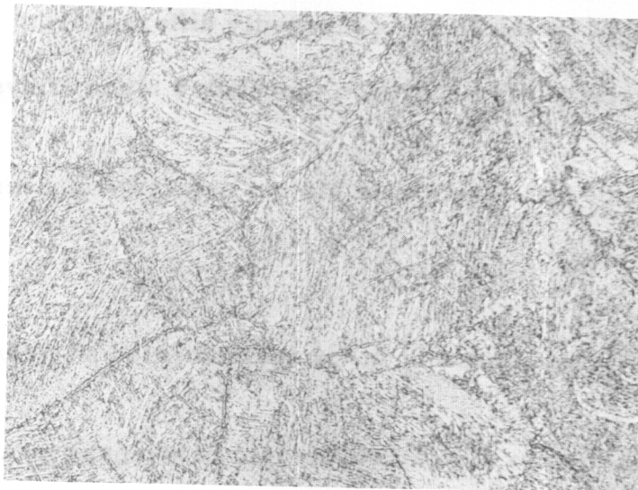
B 3 Mn COMPLEX VACUUM ANNEALED AT 1380° F (750°C) WATER QUENCH AGED 24 HRS AT 895° F (480°C)
