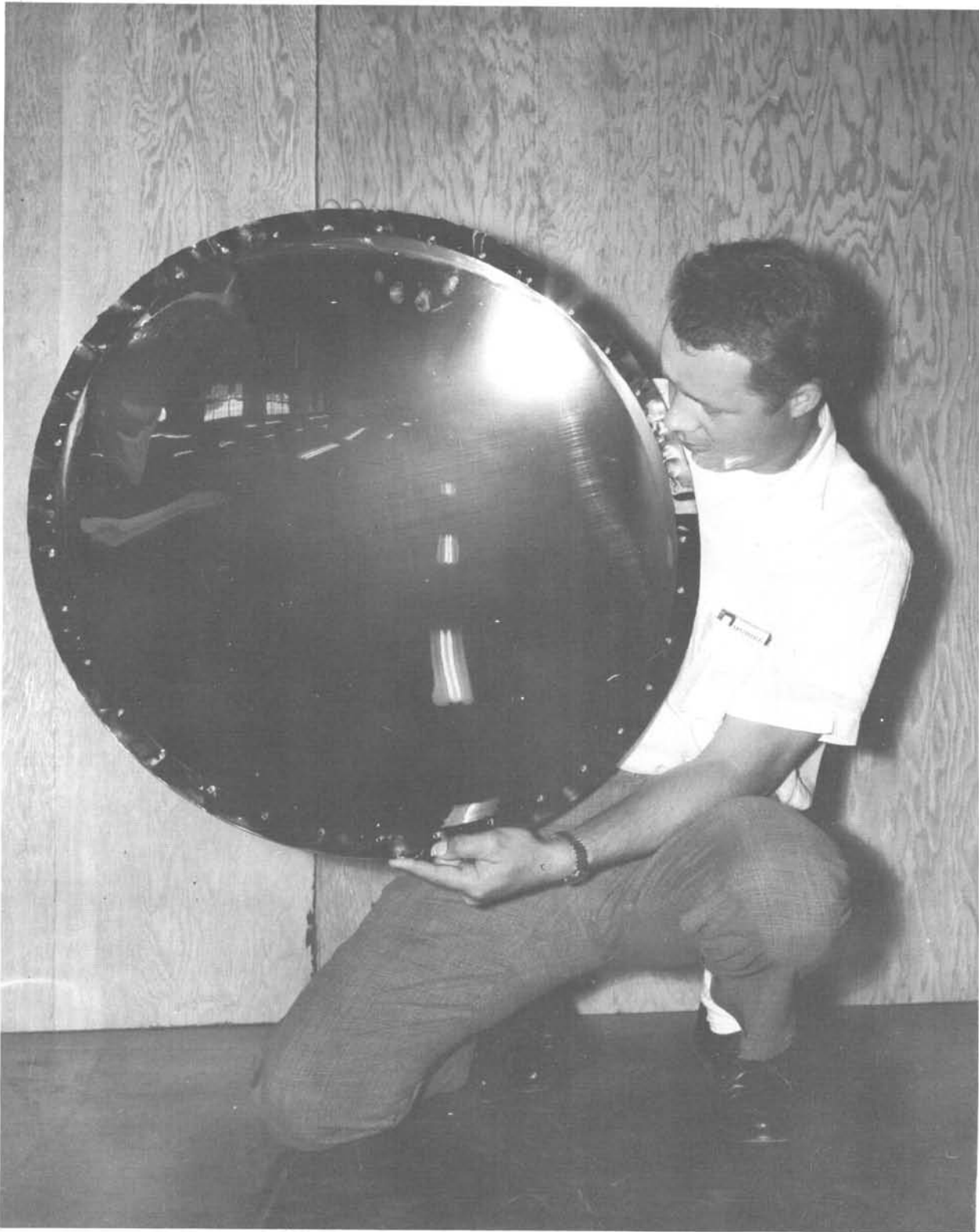
FIGURE 4 - VACUUM CURED 2 FT SOLAR COLLECTOR MODEL
