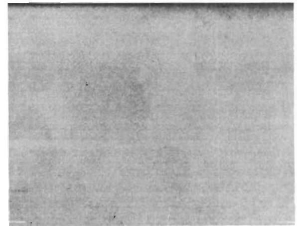
Figure 54. As-Extruded Surface of Pressed and Sintered Tungsten-3 Percent Molybdenum Extrusion 33 (Billet Code SW11) (Magnification 1-1/2X)
