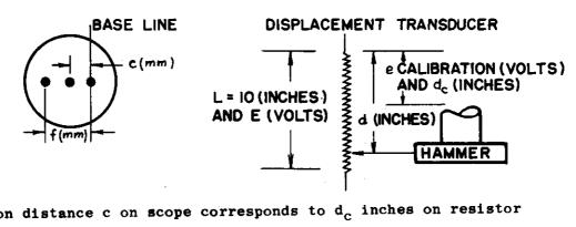
Calibration distance c on scope corresponds to  $d_{c}$  inches on resistor and distance f on scope corresponds to d inches on resistor.
