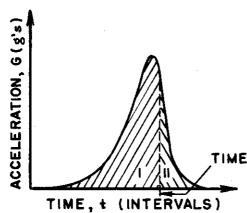
Successive values of acceleration are obtained from the smoothened velocity-time curve.
