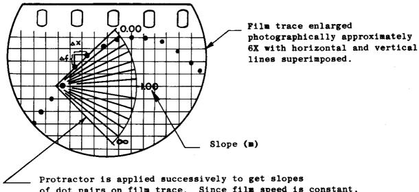
Protractor is applied successively to get slopes of dot pairs on film trace. Since film speed is constant,  $\triangle x$  is constant. Then,  $\triangle f = m \cdot \triangle x$  and substitution is made in equation (2), Figure 9, to get velocity.
