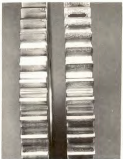
FIGURE 4. 440-C (LEFT) VS BERYLLIUM COPPER (RIGHT) 1 HR, 1000 LB/IN., 6250 RPM
