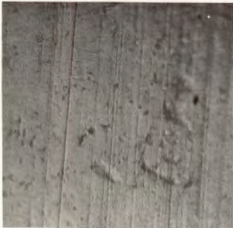
FIGURE 18. BALL BEARING RACE, 220X, N_2O_4 SUBMERGED, 4-1/2 HR, 6500 RPM, 330-LB THRUST, EDGE OF LOAD TRACK ON LEFT
