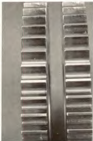
FIGURE 5. 9310 VS 9310, 15 MIN, 500 LB/IN., 6250 RPM, 1 HR, 1000 LB/IN., 6250 RPM
