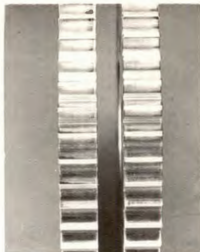
FIGURE 2. 440-C VS 440-C, 1 HR, 1000 LB/IN., 6250 RPM
