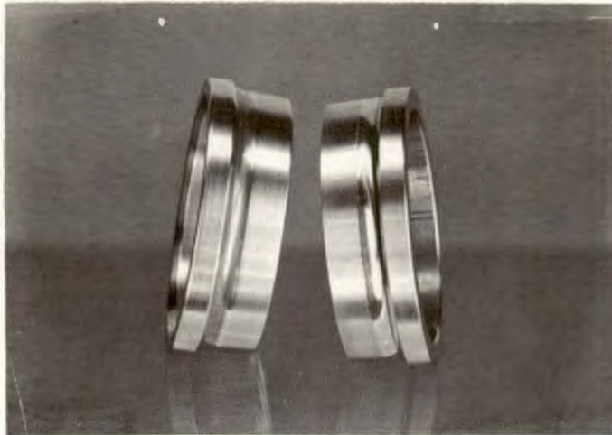
FIGURE 17. RIGHT INNER RACE, N_2O_4 , 4-1/2 HR, 6500 RPM, 330-LB LOAD
