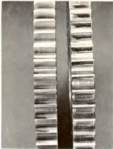
FIGURE 7. 9310 (LEFT) VS BERYLLIUM COPPER (RIGHT), 1 HR, 1000 LB/IN., 6250 RPM
