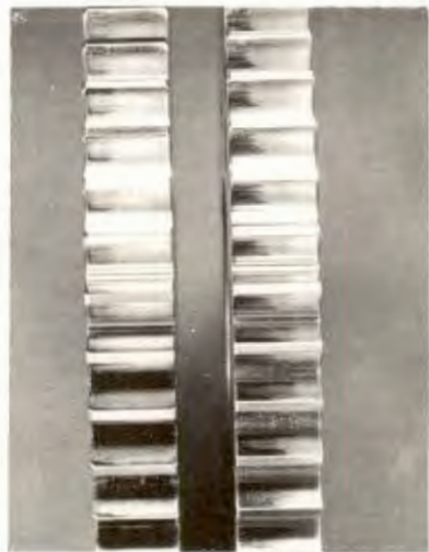
FIGURE 6. NITRALLOY 135M (LEFT) VS 9310 (RIGHT), 1 HR, 1000 LB/IN., 6250 RPM
