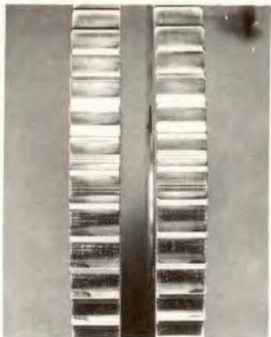
FIGURE 1. NITRALLOY 135M VS NITRALLOY 135M, 1 HR, 1000 LB/IN., 6250 RPM
