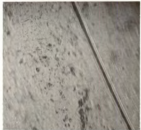
FIGURE 19. BALL BEARING BALL, 220X, N_2O_4 SUBMERGED, 4-1/2 HR, 6500 RPM, 330-LB THRUST
