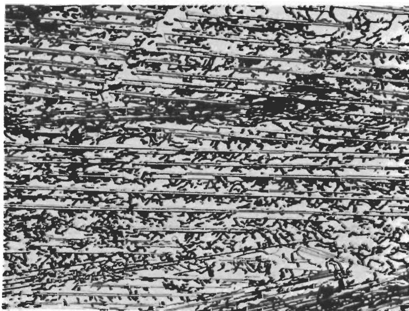
Figure 21. W-C (33.5 At% C), Quenched at \sim 100^\circ\text{C} per X250 Second from 2650°C.
