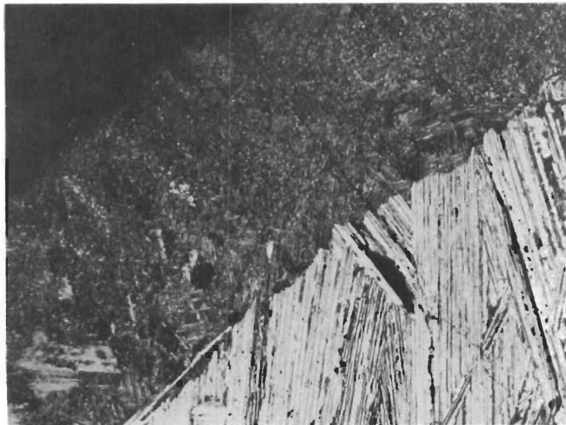
Figure 20. Diffusion Couple (W + 32 At% C)— Graphite X100 (10 Minutes at 2680°C, Radiation-Cooled)
