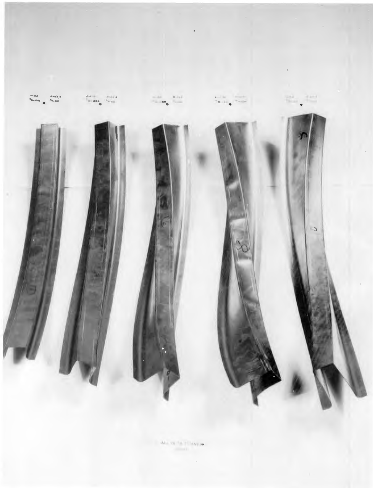
FIGURE I-59(E) TWIST BUCKLING OF LINEAR STRETCH FORMED HEEL-IN HAT SECTIONS
