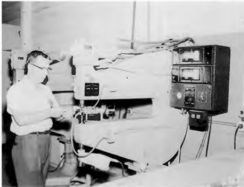
FIGURE I-20 CP450EA ZEPHYR TRIPLE ACTION COIN RAM DIMPLING MACHINE
