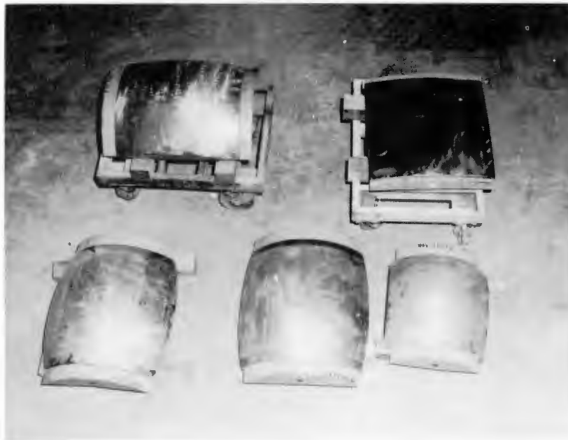
FIGURE I - 74 DOUBLE CONTOUR SHEET STRETCH DIES
