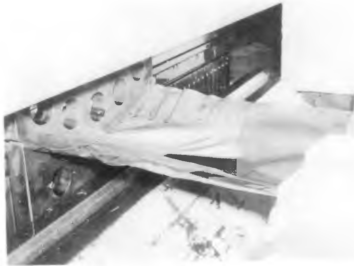
FIGURE I - 86 BUCKLING OF ANDROFORM PARTS
