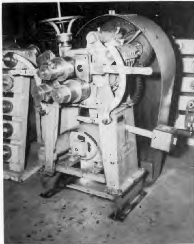
FIGURE I-60 KANE-ROACH ( 3 ROLL) ROLLING MACHINE
