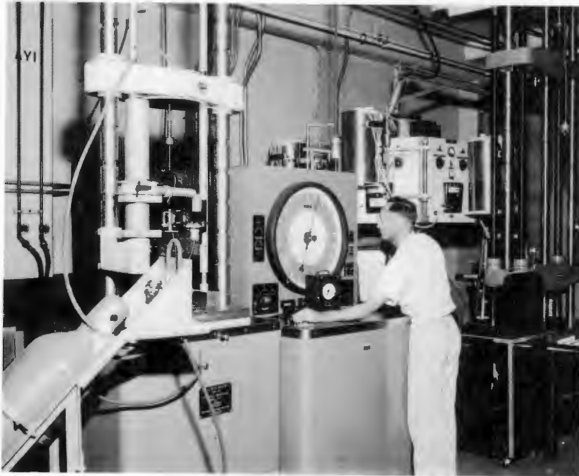
FIGURE IV-1 MODEL FGT - SR4 T/M BALDWIN TENSILE TEST MACHINE
