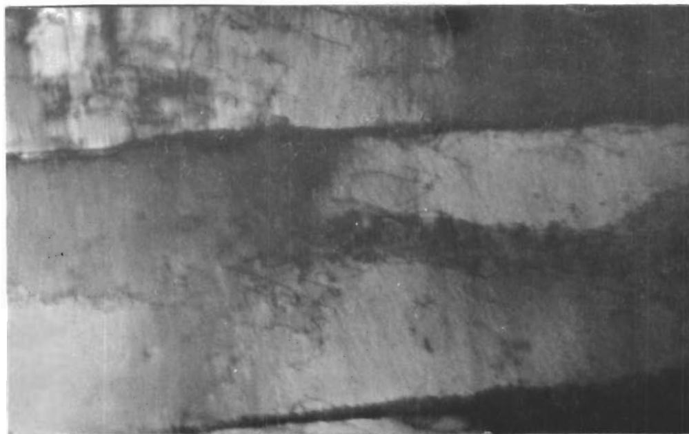
Fig. 72b - Annealed 30 minutes at 1000°C. 40,000X.
