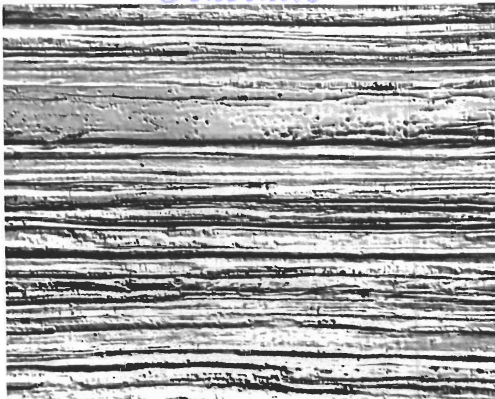
Fig. 3 - Microstructure of as-drawn tungsten (W-P4) wire.
