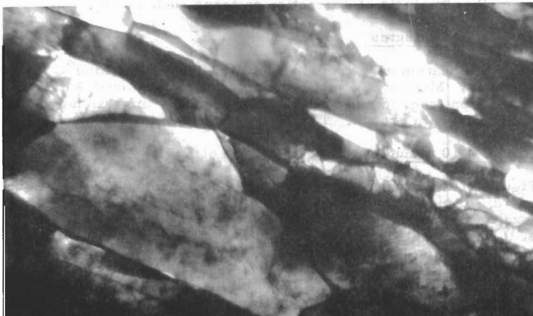
Fig. 68b - Annealed 10 minutes at 1200°C. 20,000X.
