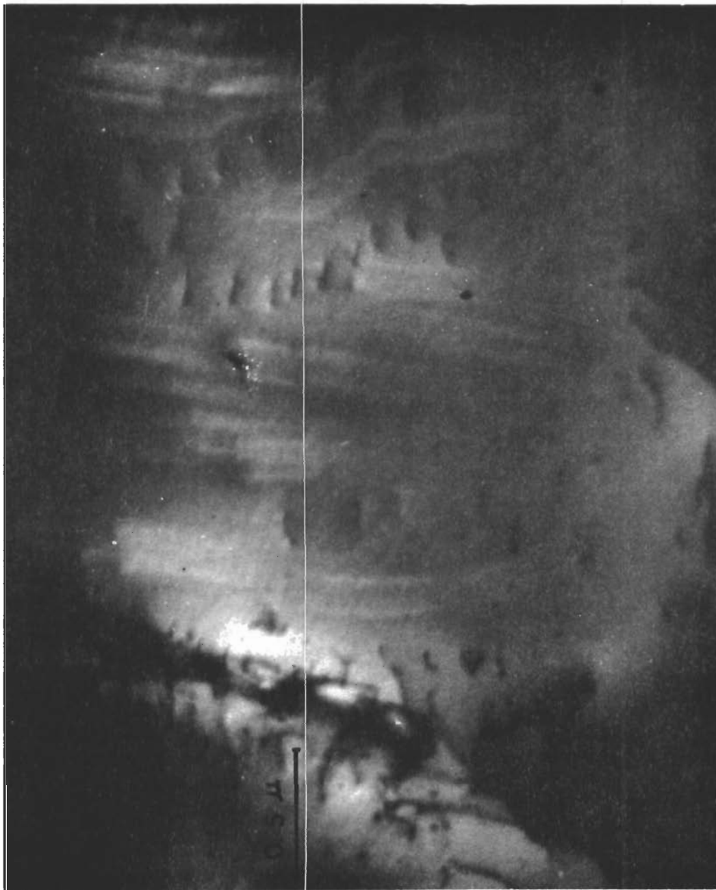
Fig. 92 - Evidence of cross-slip shown by the zigzag trail of screw dislocation.
