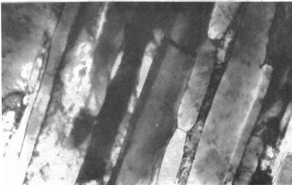
Fig. 66b - Annealed 10 minutes at 900°C. 40,000X.
