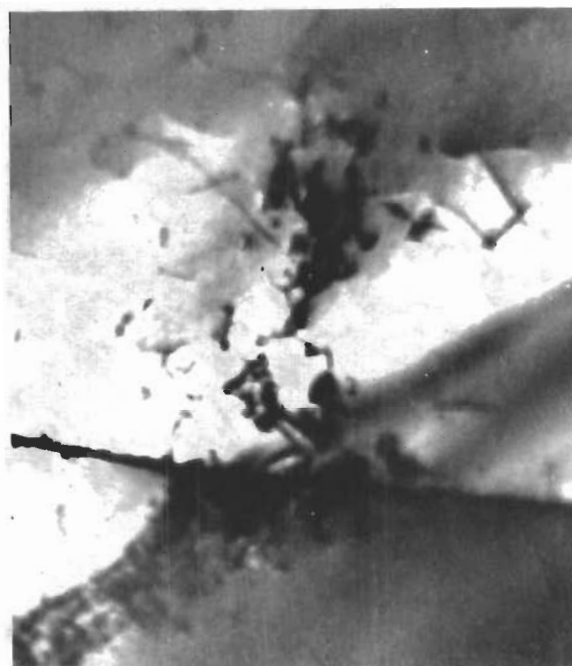
Fig. 148 -Ta-E4 strained 4.3% in strain at 293°K.
