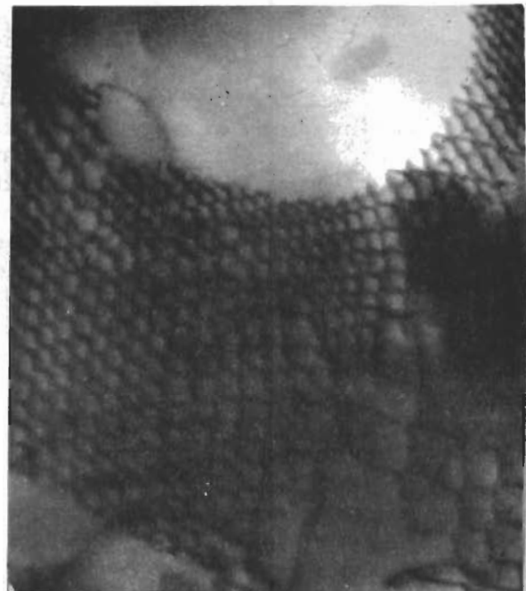
Fig. 117 - Dislocation network almost parallel to the plane of the foil in Ta-E1 annealed at 1200°C
