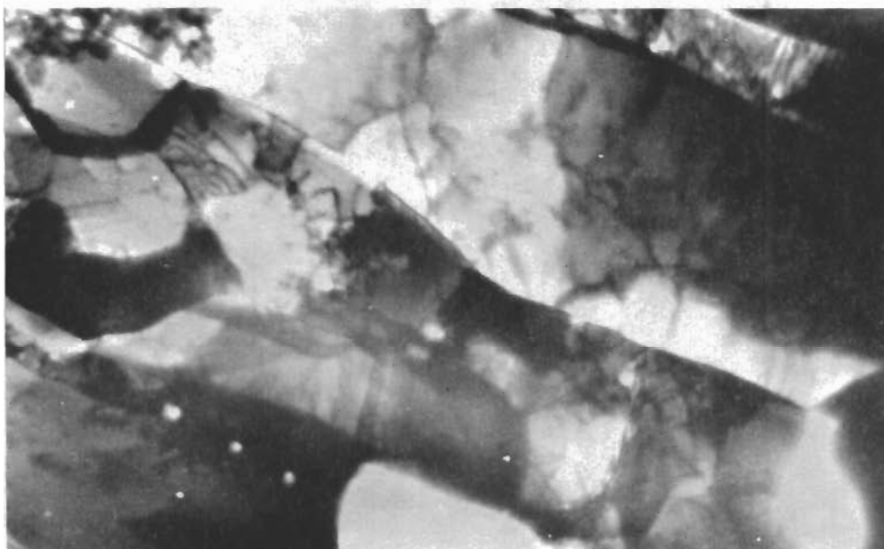
Fig. 71b - Annealed 10 minutes at 1400°C. 20,000X.
