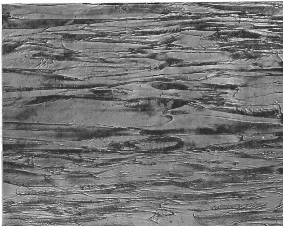
Fig. 43 - Substructure in recrystallized Ta-EI wire.
