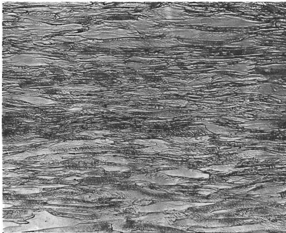
Fig. 47 - Substructure in recrystallized Ta-E3 wire.
