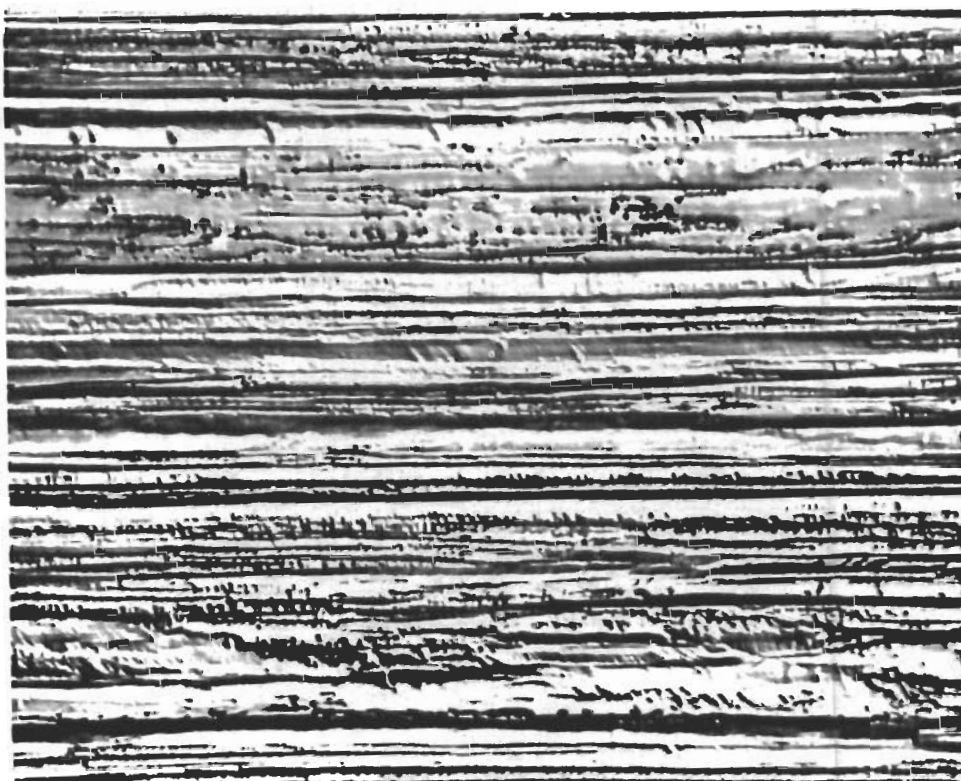
Fig. 3 - Microstructure of as-drawn tungsten (W-P4) wire.
