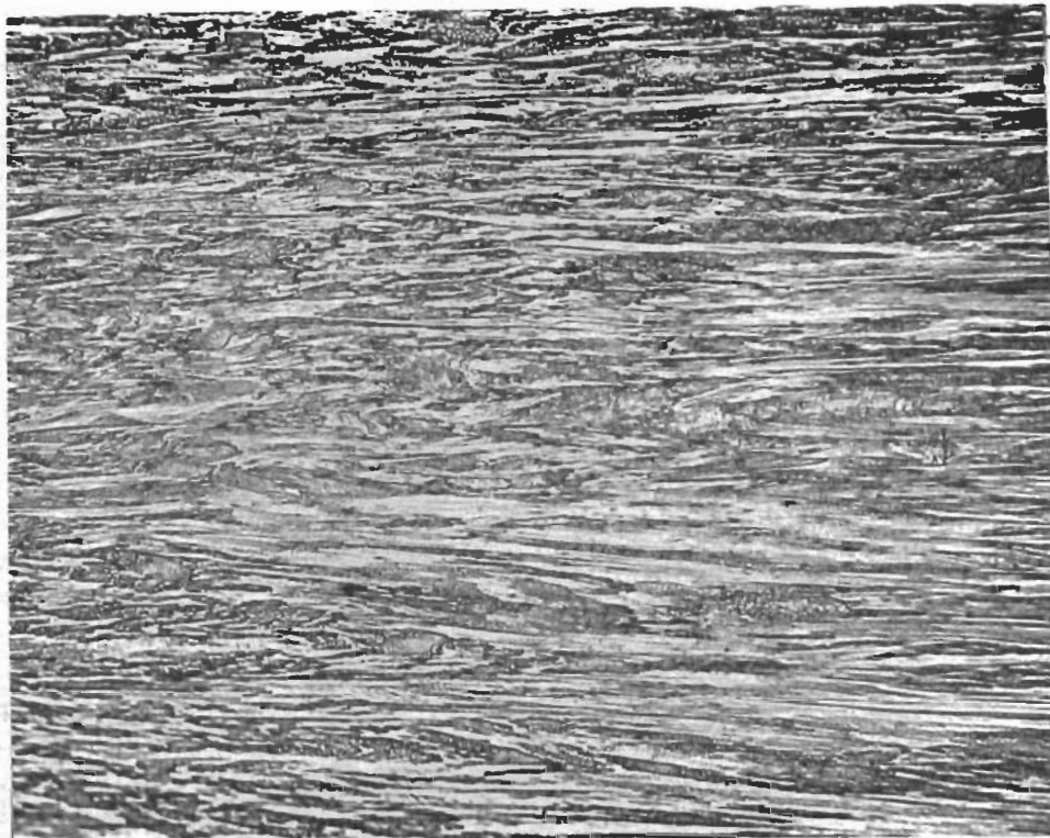
Fig. 31 Microstructure in the necked region of a tungsten (W-P4) wire tensile specimen tested at 80° in the as-drawn condition.
