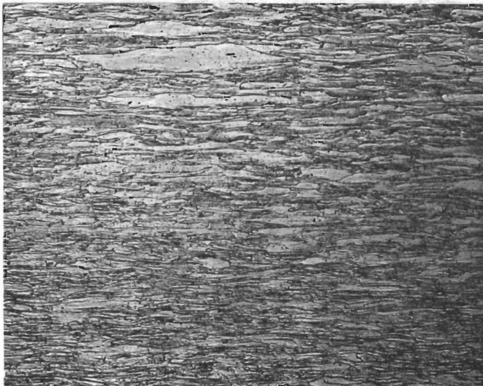
Fig. 45 - Substructure in recrystallized Ta-E2 wire.
