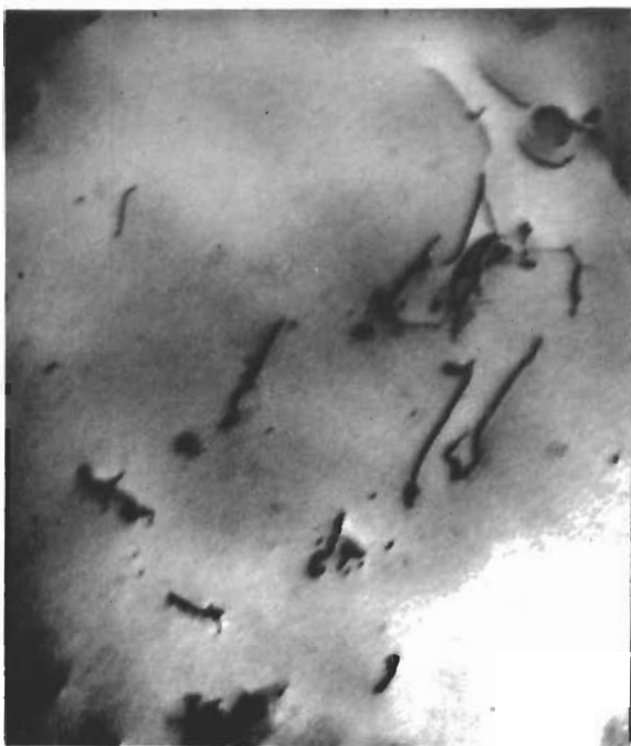
Fig. 144 - Ta-E4 strained 2.8% in strain at 293°K.
