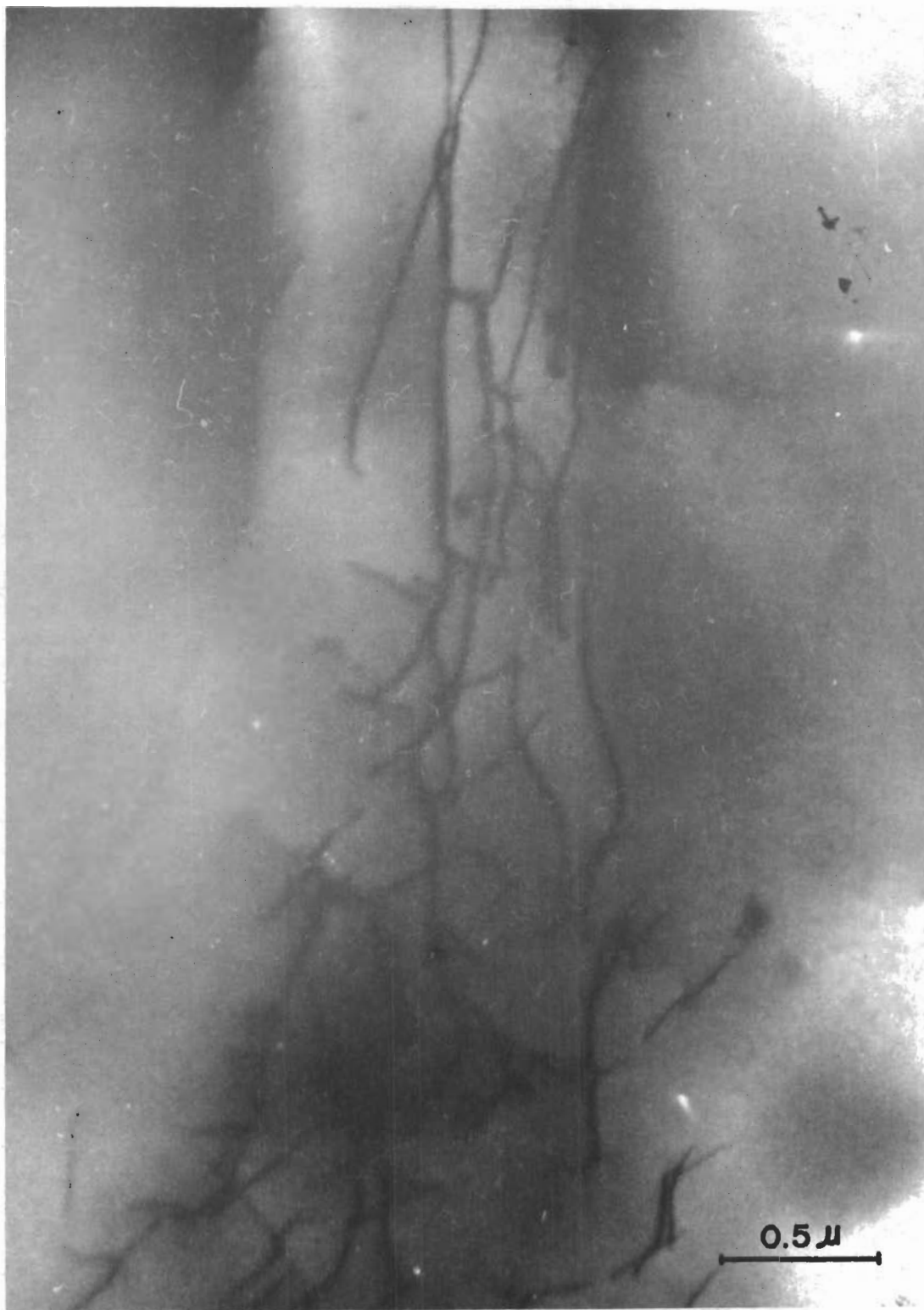
Fig. 86 - Ta-E1 annealed at 1500°C in vacuo. Note the straight dislocation lines and the poorly developed hexagons.
