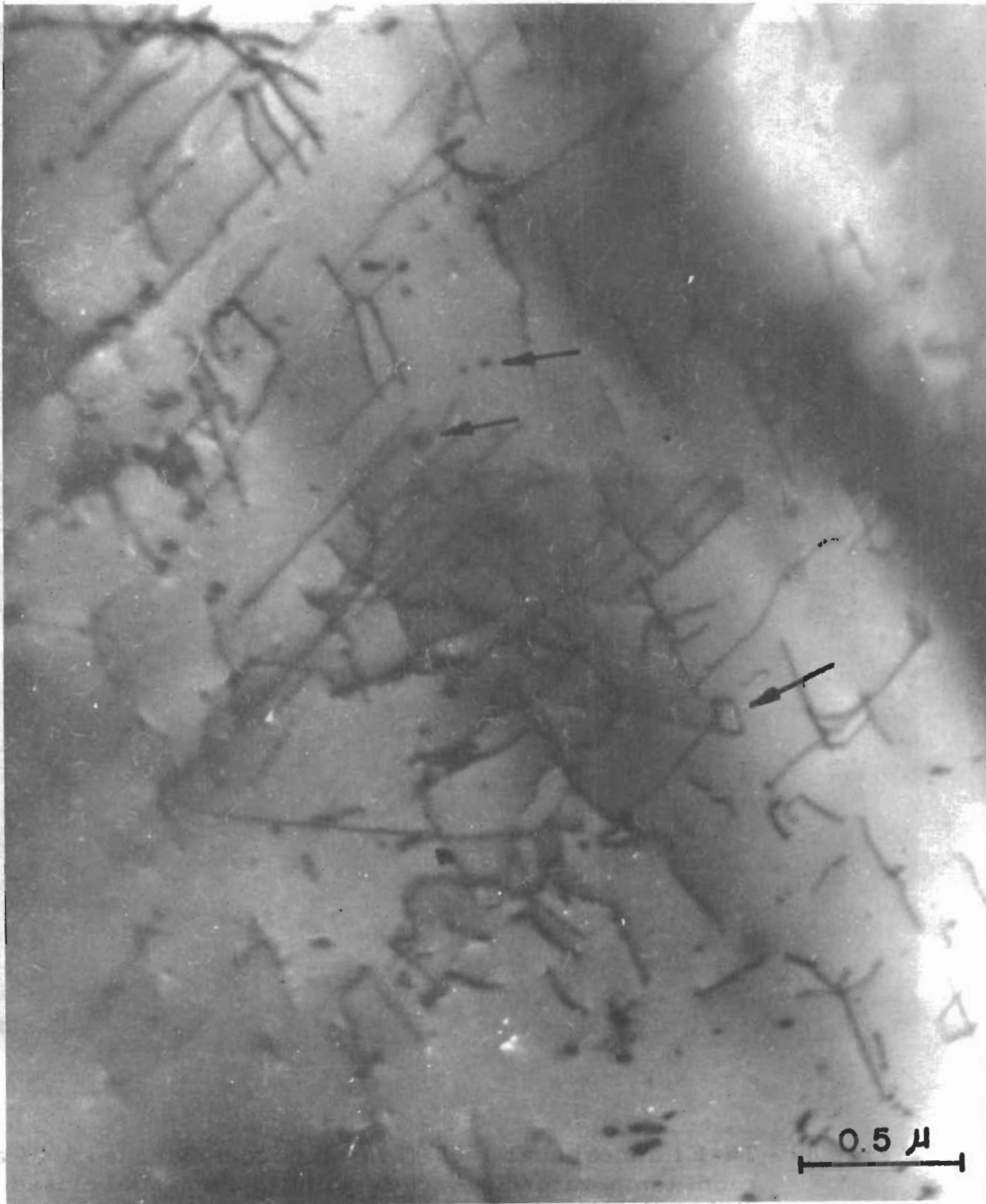
Fig. 90 - Ta-E1 annealed at 1500°C in vacuo and extended 2% at room temperature. Arrows point to cusps and closed loops resulting from cross-slip.
