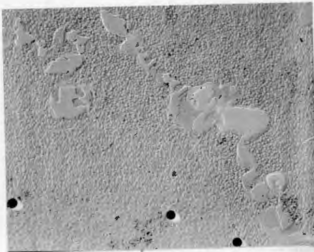
Figure 6 Udimet 500 - As Heat Treated (2150°F - 2 hr + Air Cool 1975°F - 4 hr + Air Cool 1550°F - 24 hr + Air Cool 1400°F - 16 hr + Air Cool)
