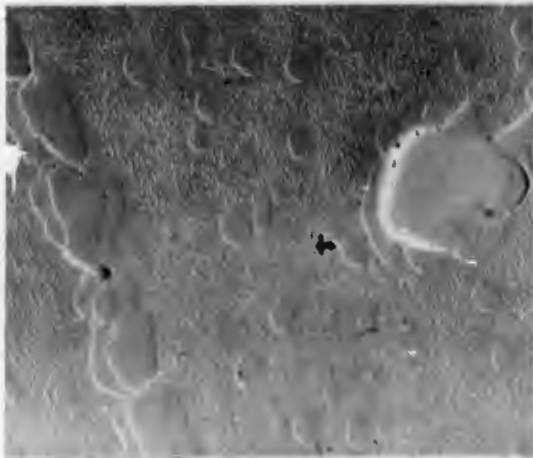
Figure 49 8200x Specimen R-79 Creep-Exposure 200 Hours at 1800°F to 1.80% Deformation
