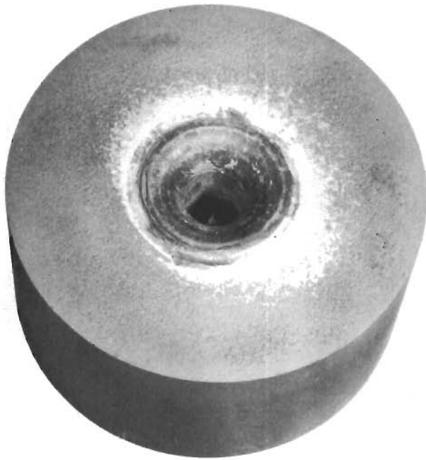
0.030 in. ZrO_2 coating in steel
