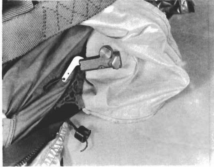
Figure 12. The Flotation Triggering Mechanism
