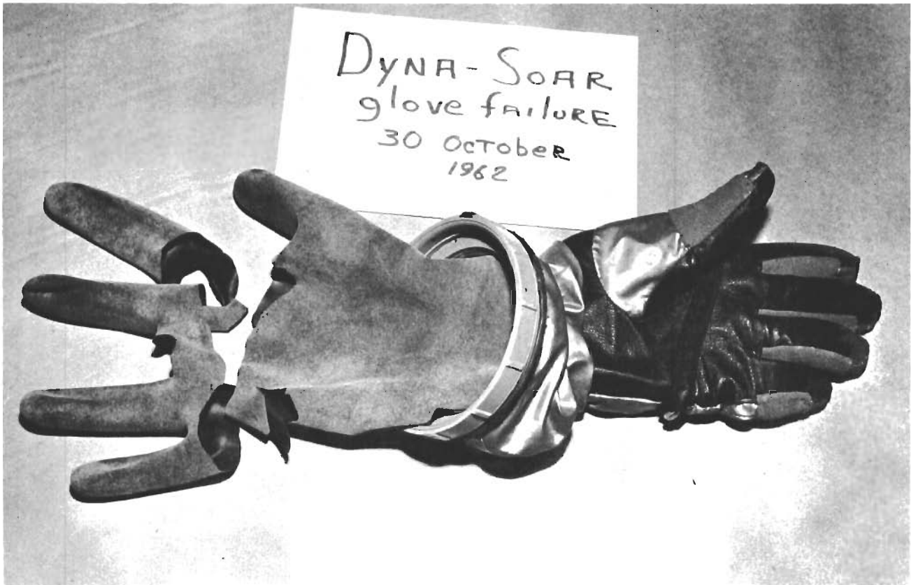
Figure 30. Glove Bladder Failure
