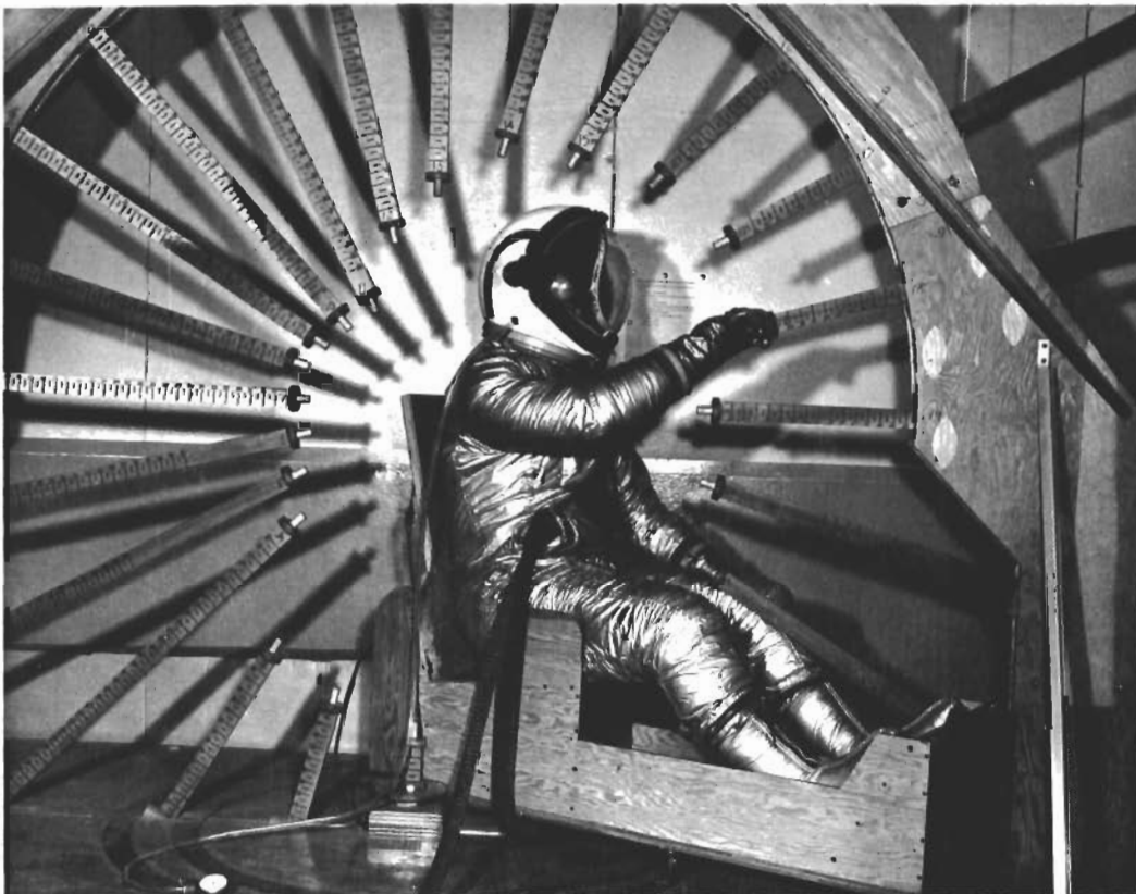
Figure 16. Arm Reaching Measuring Device
