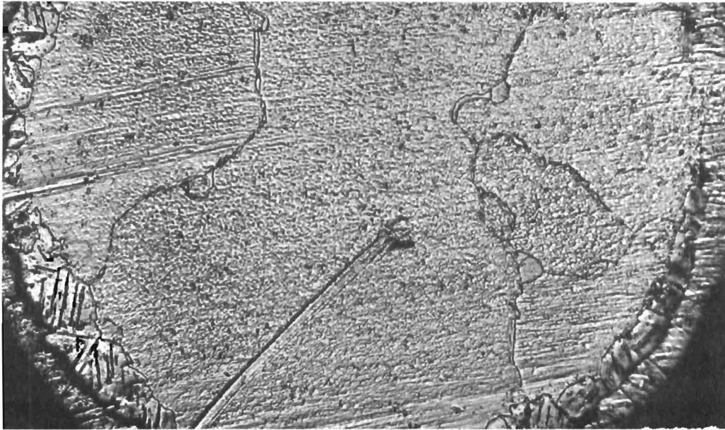
Fig. 48a. Photomicrograph of Carbided Tungsten Specimen Provided with Scratch - 200X
