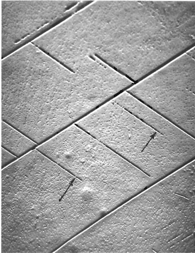
Fig. 16 Deformation Twins in Tungsten Single Crystals as Revealed by Polishing and Etching - 500X
