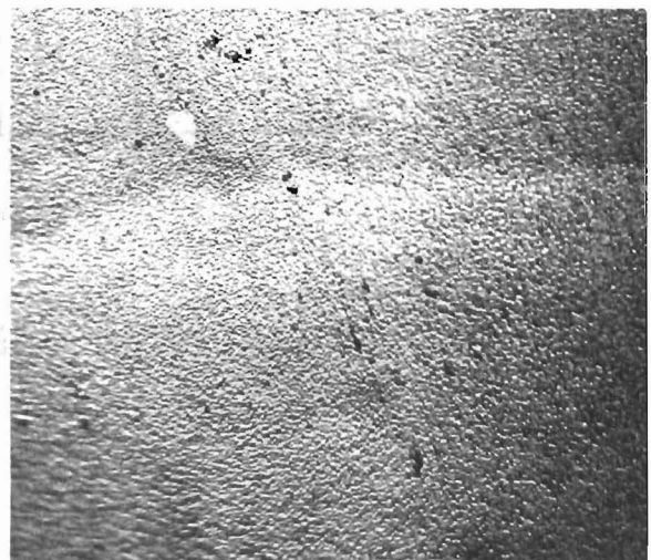
Fig. 53 Tungsten Single Crystal after Vacuum Anneal at 2200°C, 6 hrs. following anneals per Figs. 50, 51 and 52; 600X
