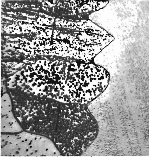
Fig. 90 W-.35% Ta, 80% R.A. after 1/2 hour at 1500°C - 500X
