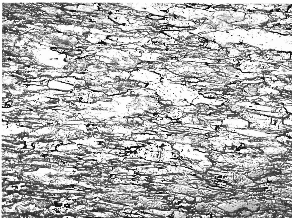
Fig. 100 W + 0.38% TaC - as swaged % R.A. at 1650°C- 1700°C. Direction of working - horizontal - 250X
