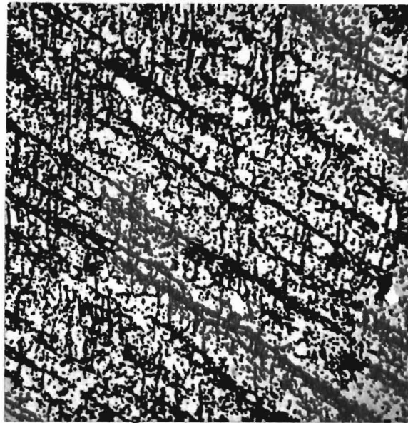
Fig. 92 W-.35% Ta, 30% R.A. after 1/2 hour at 1500°C - 500X
