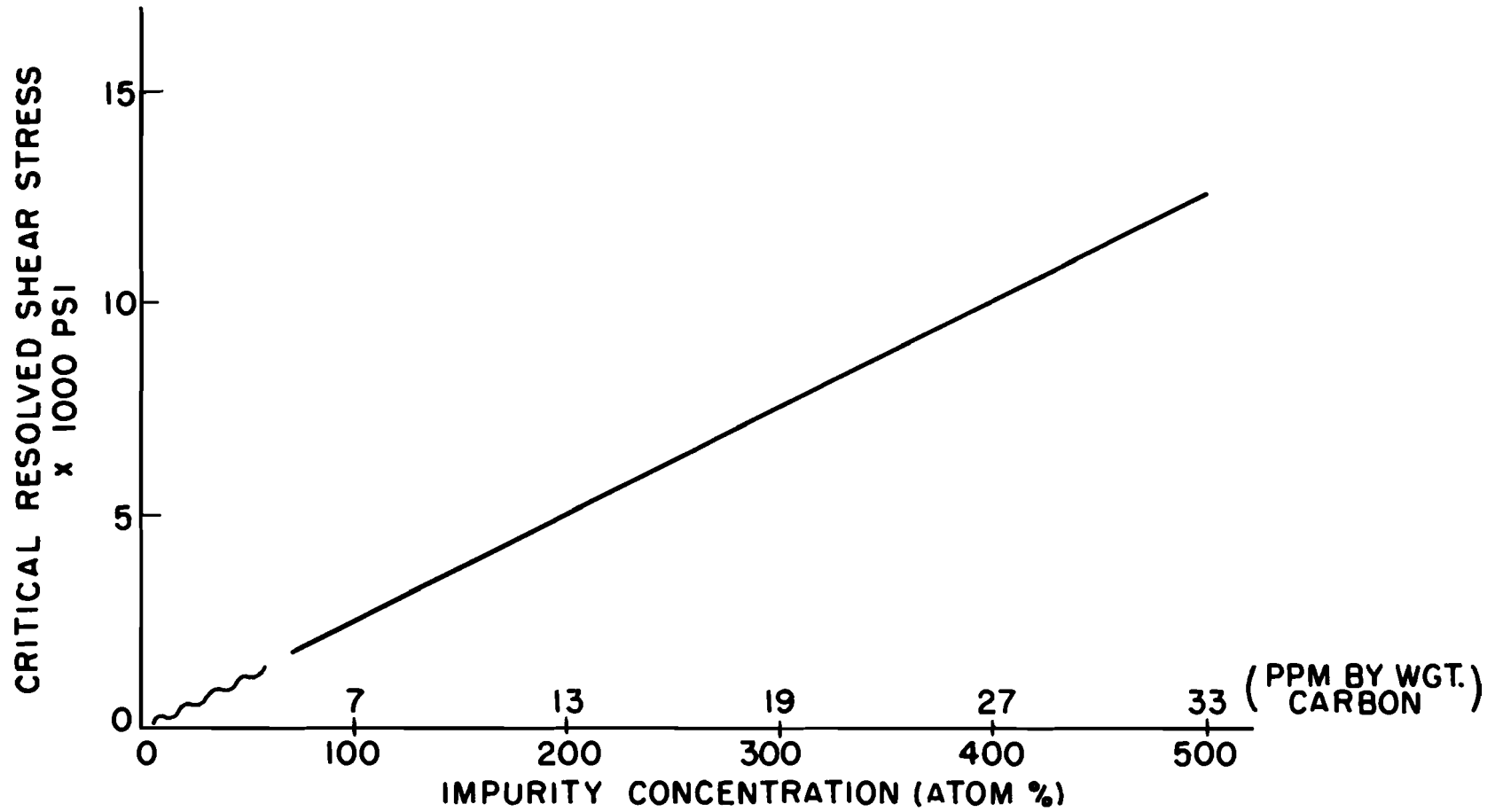
FIG. 31 CRITICAL RESOLVED SHEAR STRESS AS A FUNCTION OF IMPURITY CONCENTRATION PER EQUATION:
