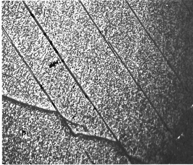
Fig. 22 Twins on Fracture Surface of Single Crystal Tensile Specimen Tested at 300°C - 150X
