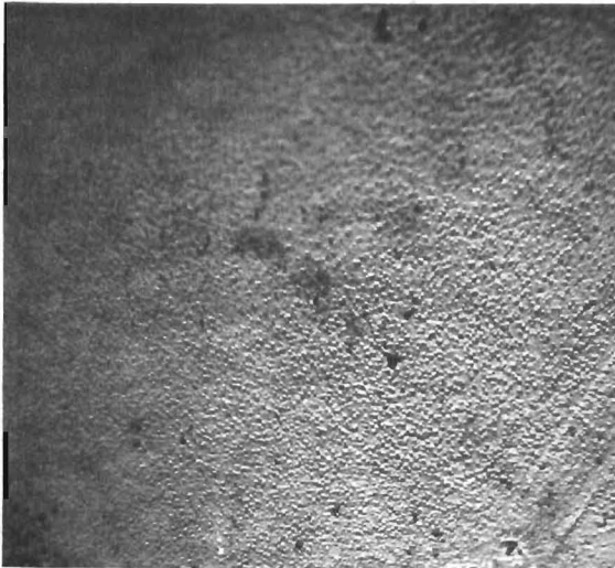
Fig. 50 Tungsten Single Crystal after Vacuum Anneal at 2200°C, 5-1/2 hrs.; 600X
