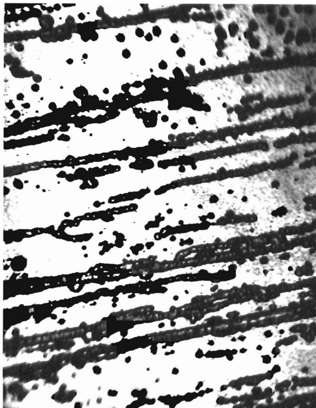
Fig. 57 Single Crystal Tungsten No. UC-2 as Rolled 80-90% R.A. - 1000X
