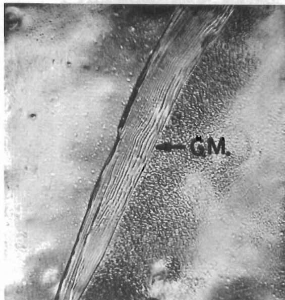
Fig. 59 Single Crystal Tungsten No. UC-2 Rolled 80-90% R.A., Annealed for 3 Hrs. at 1100°C - 100X
