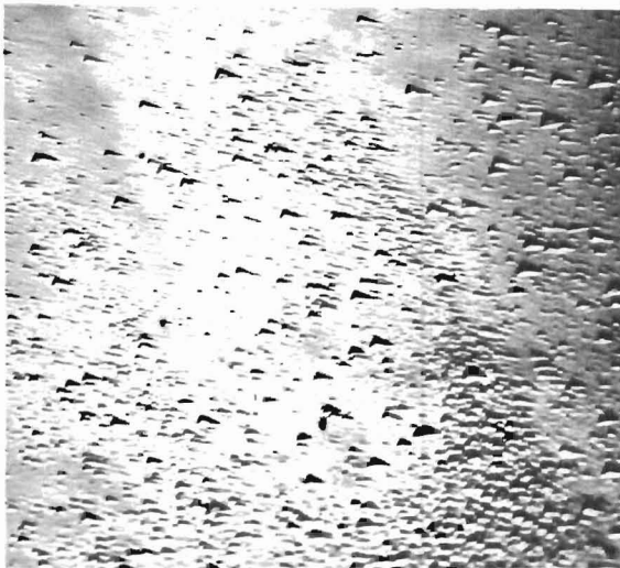
Fig. 52 Tungsten Single Crystal after Precipitation Anneal at 600°C, 7-1/2 hrs. following anneals per Figs. 50 and 51; 600X
