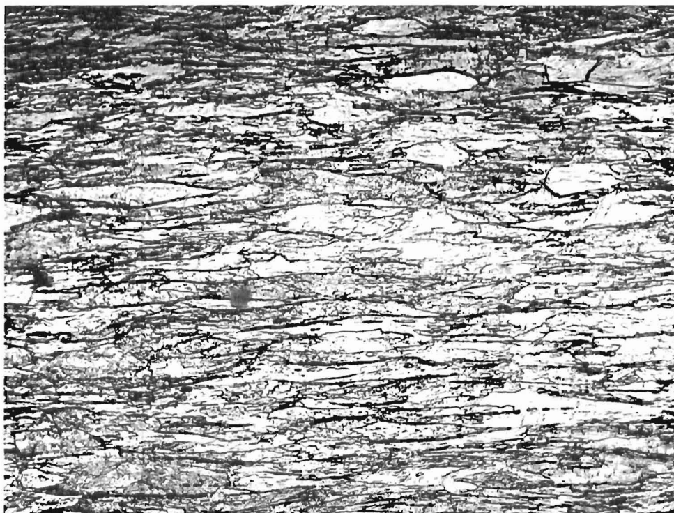
Fig. 100 W + 0.38% TaC - as swaged % R.A. at 1650°C- 1700°C. Direction of working - horizontal - 250X
