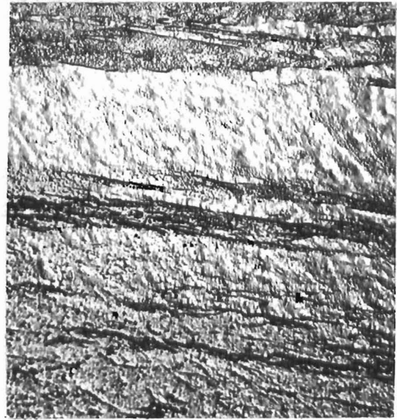
Fig. 91 W-5% Ta, 80% R.A. after 1/2 hour at 1500°C - 500X
