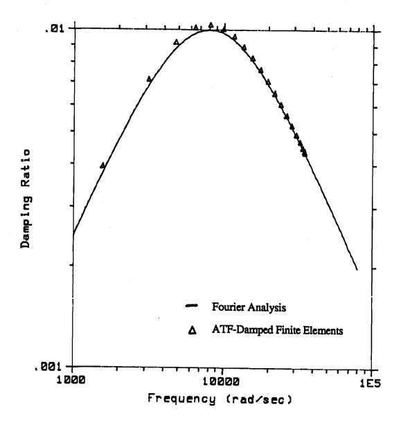
Figure 4: Damping versus Frequency for 20 ATF-Damped Rod Finite Elements and Fourier Analysis
