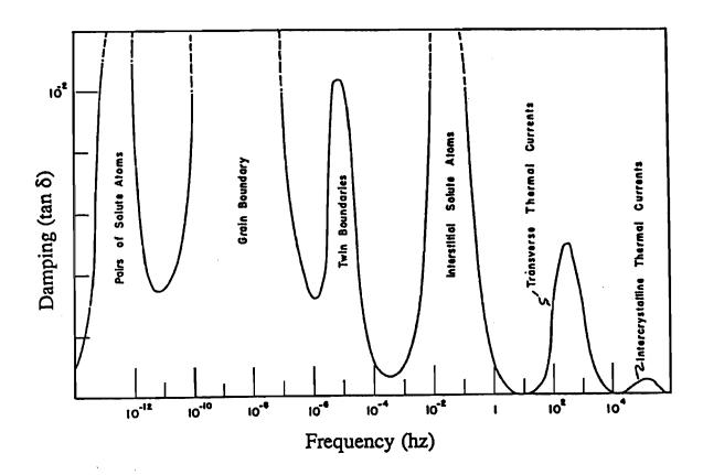
Figure 1: Typical Frequency-Dependence of Material Damping (from [Zener, 1948])
