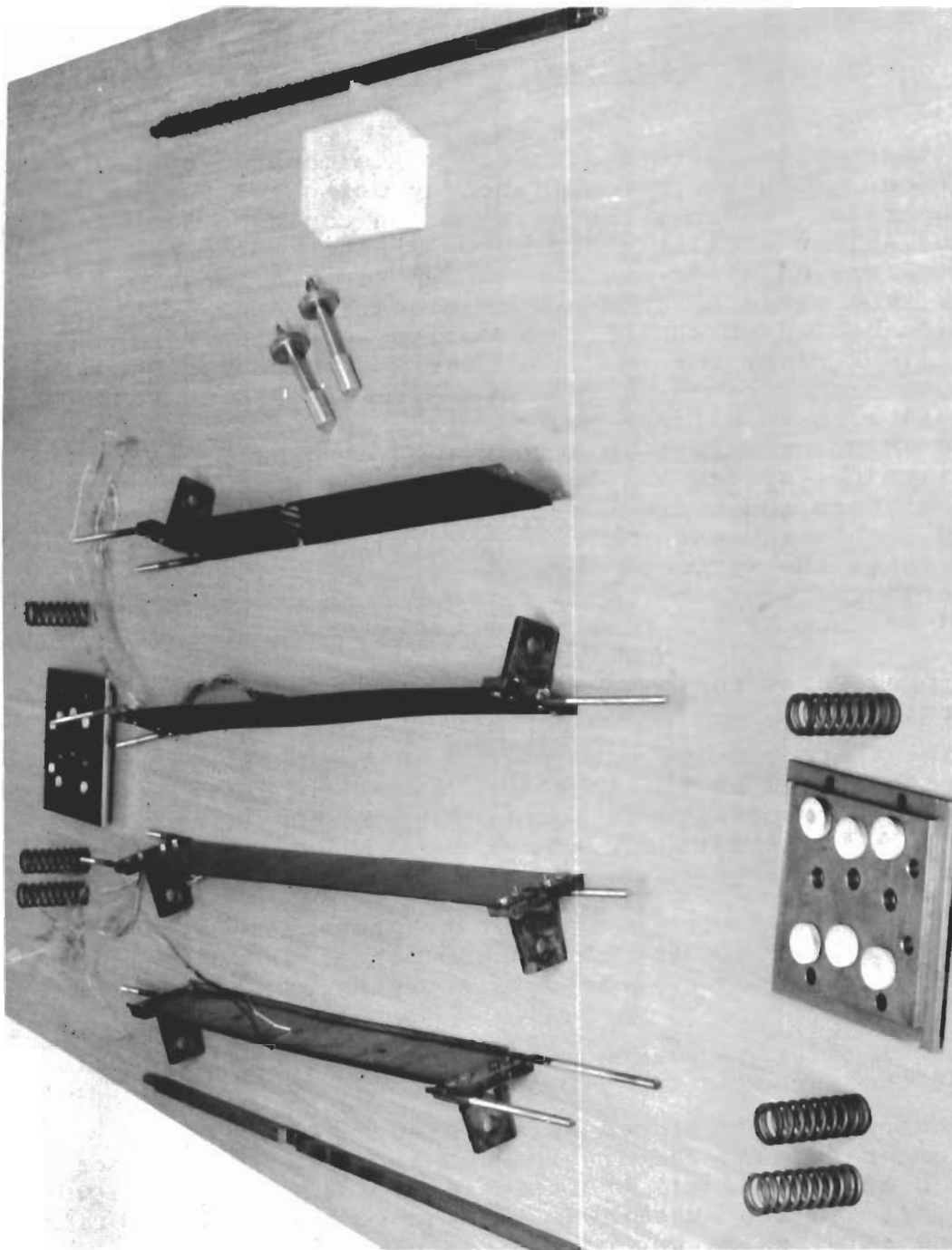
Figure 10 View of Test Assembly, Components, Test Surfaces, Guard Plates, and Thermopiles
