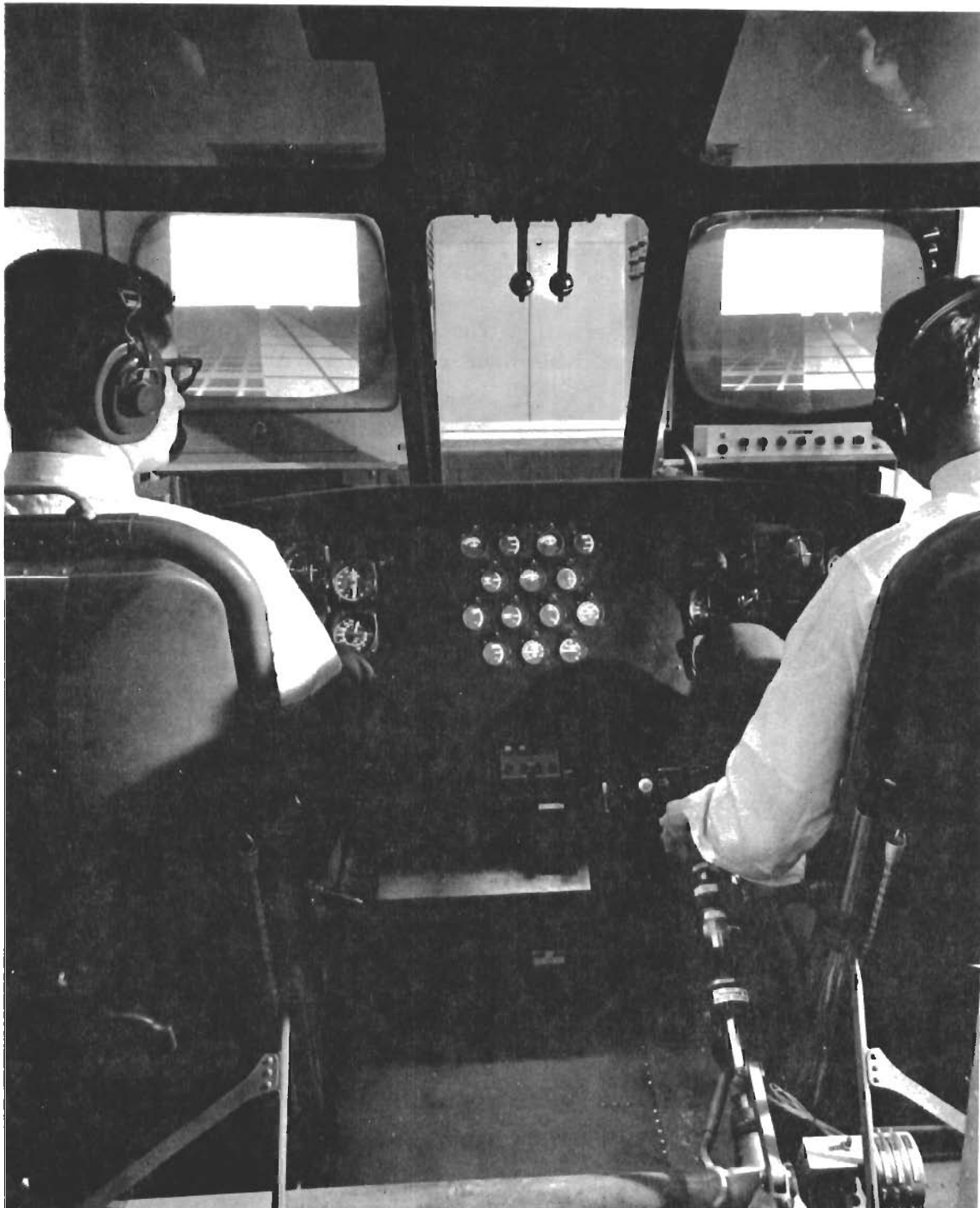
Figure 1. Photograph of Interior of V/STOL Aircraft Flight Simulator
