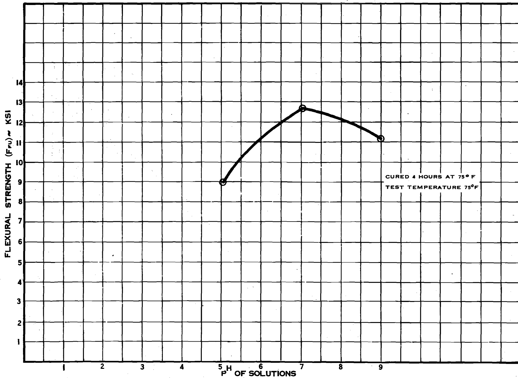
Figure 19 Effect of pH Solutions on Flexural Strength of Formula A Resin System
