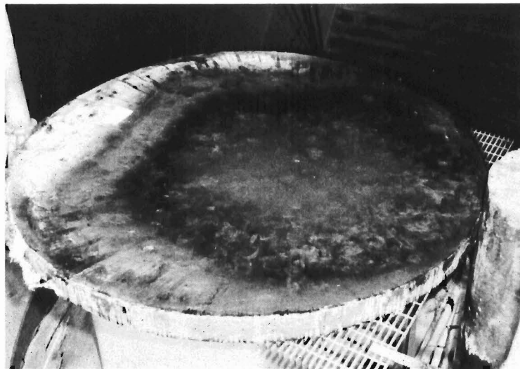
Figure 13 Typical 9-Ft Diameter RTD Jet Engine Test Specimen (Filled Polyester and Fiberglass Before, During, and After Exposure)
