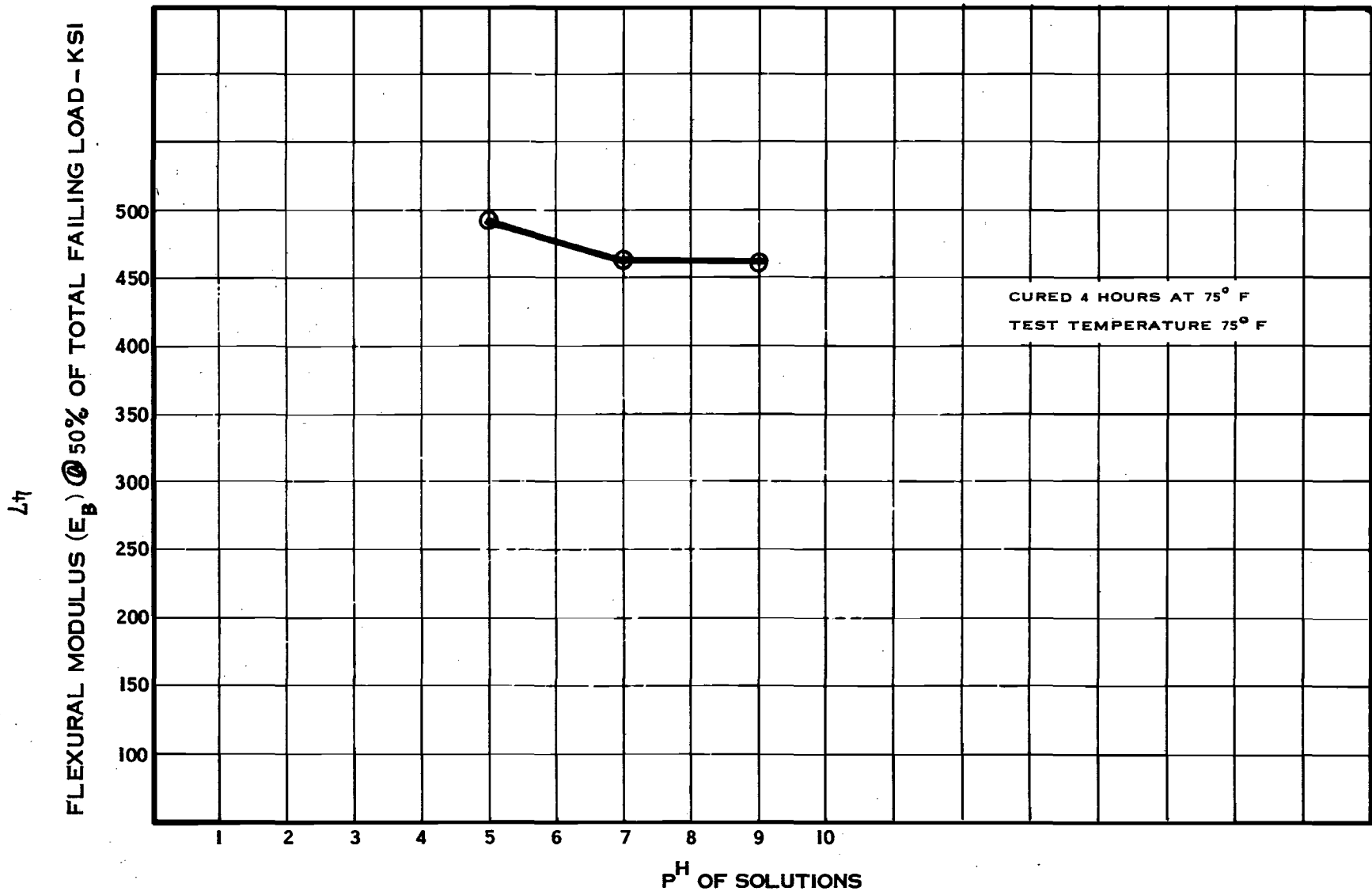
Figure 20 Effect of pH Solutions on Flexural Modulus of Formula A Resin System
