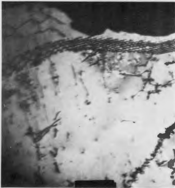
Figure 5. TaE4 Annealed 1000°C, Deformed 6.7% in Tension X40,000
