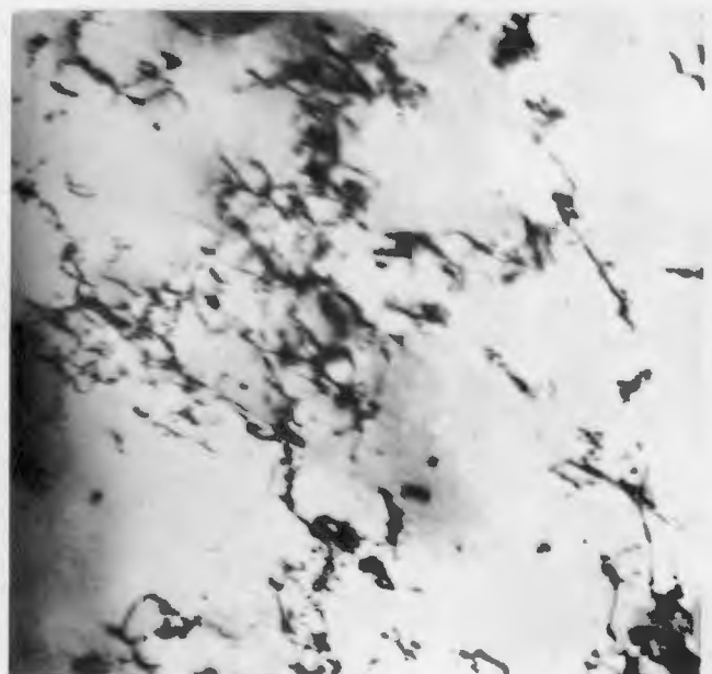
Figure 4. TaE4 Annealed 1750°C Deformed 10.0% in tension X40,000
