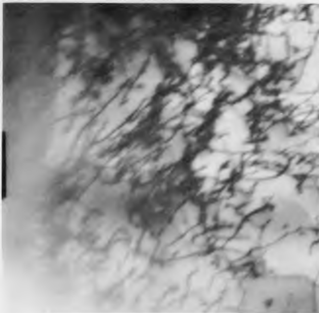
Figure 3. TaE1 Annealed 1200°C, Deformed 12.2% in tension. X40,000
