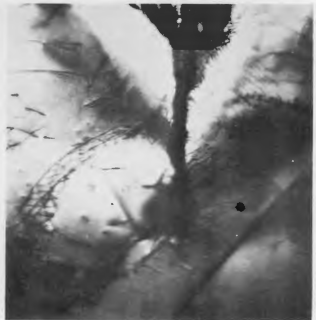
Figure 6. TaE4 Annealed 1000°C, Deformed 6.7% in Tension X40,000
