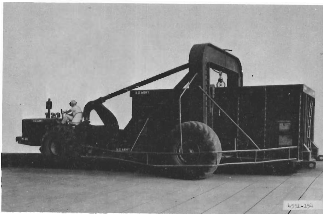
Figure 1. Test load vehicle
