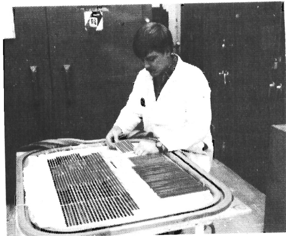
Figure 2. Constrained Layer Damper Fabrication
