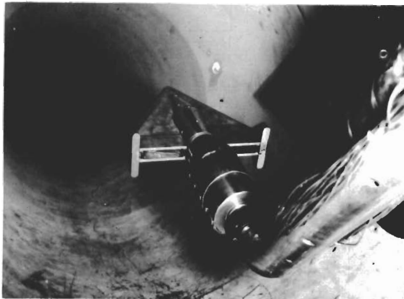
Figure 28. Photograph of Winged Re-entry Configuration in the AEDC 50-Inch Mach 8 Tunnel
