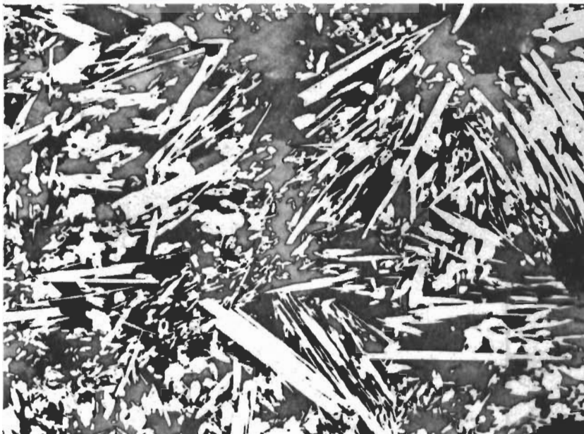
Figure 11. Hf-B (30 At% B), Quenched with Approximately 20°C per Second from 1910°C. X500
