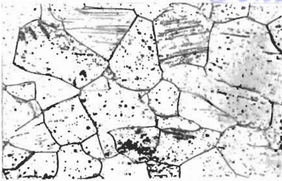
Neg. No. 22777 (a) No addition grain dia. = 3.5 \times 10^{-3} in.
