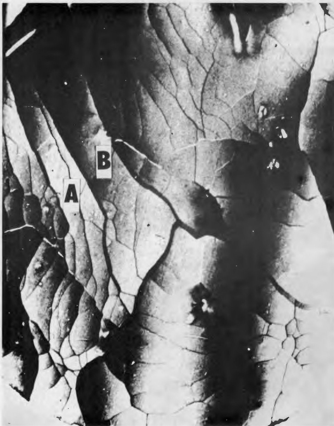
Fig. 10—X-ray oscillation reflection micrograph of tungsten single crystal grown by arc fusion. Effective focal spot size 40\mu . Disclosure of macroscopic and microscopic substructure. Magnification 40 x.
