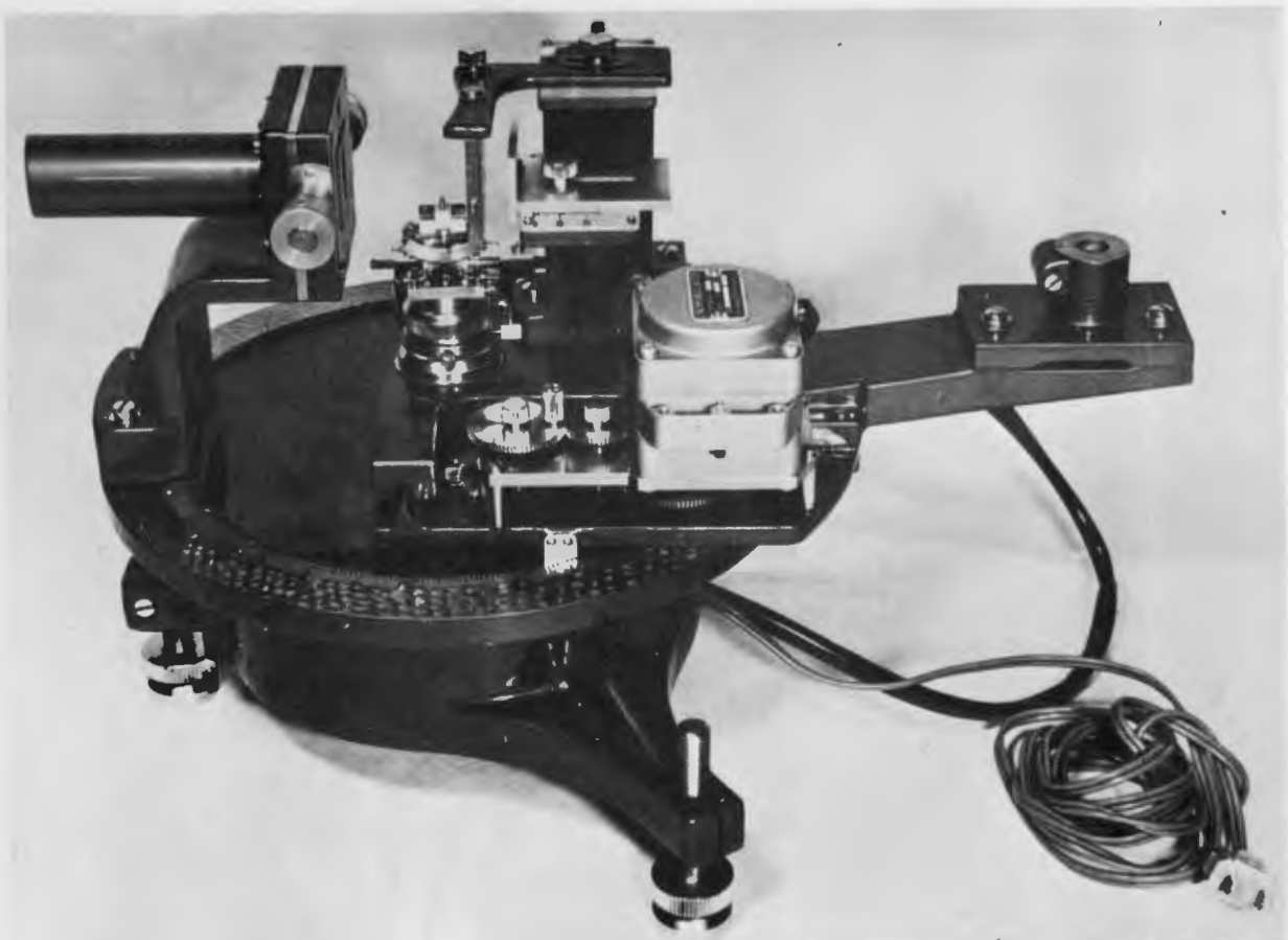
Fig. 14--Commercial Lang camera for x-ray diffraction topography (courtesy of Rigaku-Denki Co.).
