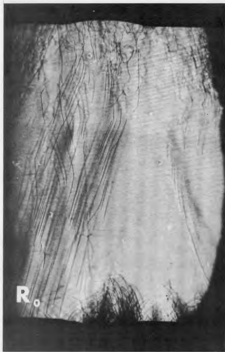
Fig. 17--R and R 0 image of germanium wafer showing dislocations and segregation of arsenic. (220) reflection. 12 x. (After Schwuttke 21 ).
