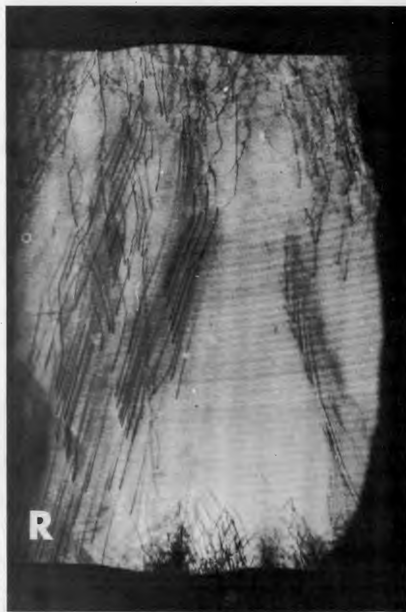
Fig. 17--R and R 0 image of germanium wafer showing dislocations and segregation of arsenic. (220) reflection. 12 x. (After Schwuttke 21 ).
