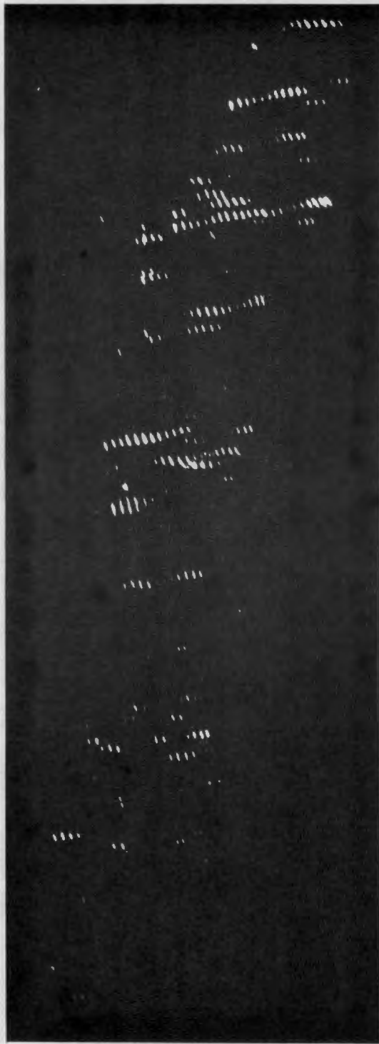
Fig. 8--Detailed view of (422) reflection of multiple-exposure diagram exhibiting multi-modal intensity distribution curves typical of subgrain structure. Al 99.95% pure, 96% reduced and annealed 1 hour at 300° C. Specimen rotation interval 4'.
