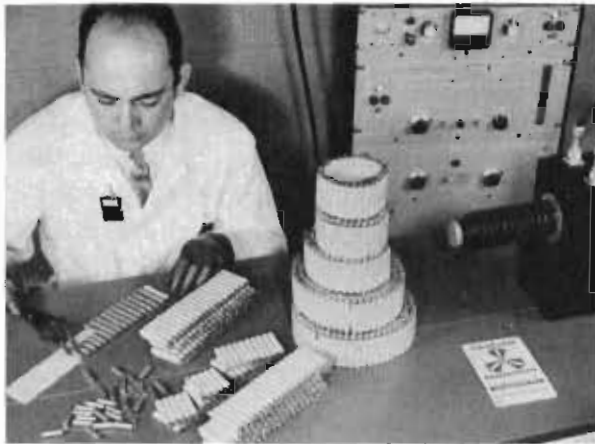
Figure 39. Low Activity Assembly of Cobalt 60 Configuration
