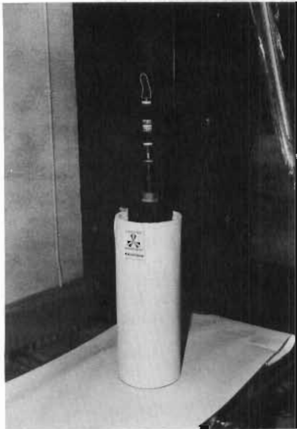
Figure 32. Location of Albedo Measurement over Source Well
