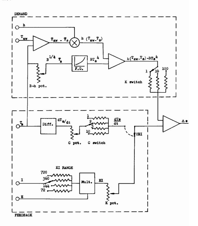
Figure 5. Schematic Diagram for Power Feedback and Derivative Modes
