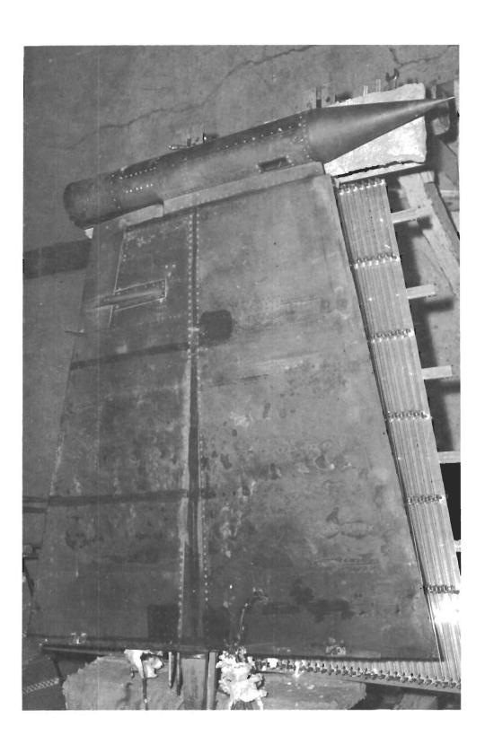
Figure 3. X-7A Wedge-Shaped Wing
