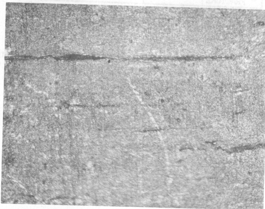
FIG. 82 CRACK DEVELOPMENT IN A Cd-PLATED BEND SPECIMEN. TESTED AT SLOW SPEED
