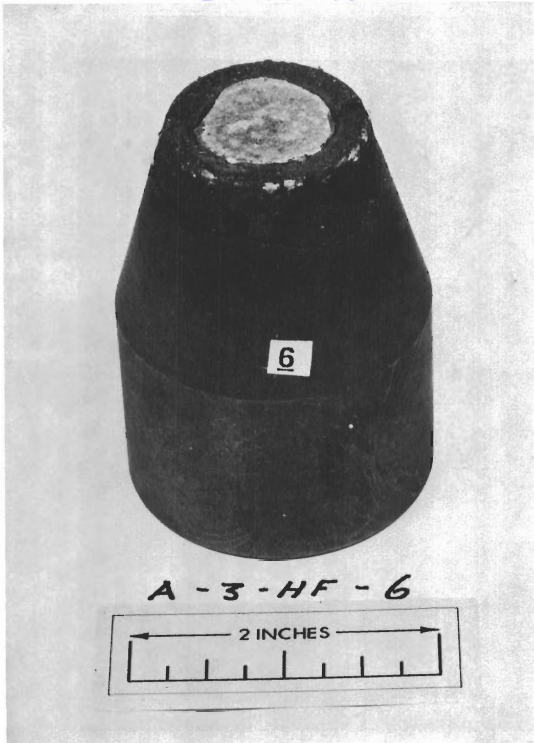
Figure 63. Post Test View of Sample Tested in Ten Megawatt Arc Facility (#18420C).
