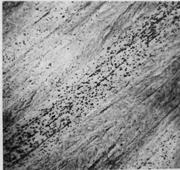
Fig. 16. Carbon extraction replica showing carbide precipitation along deformation band in ausformed steel 18.
