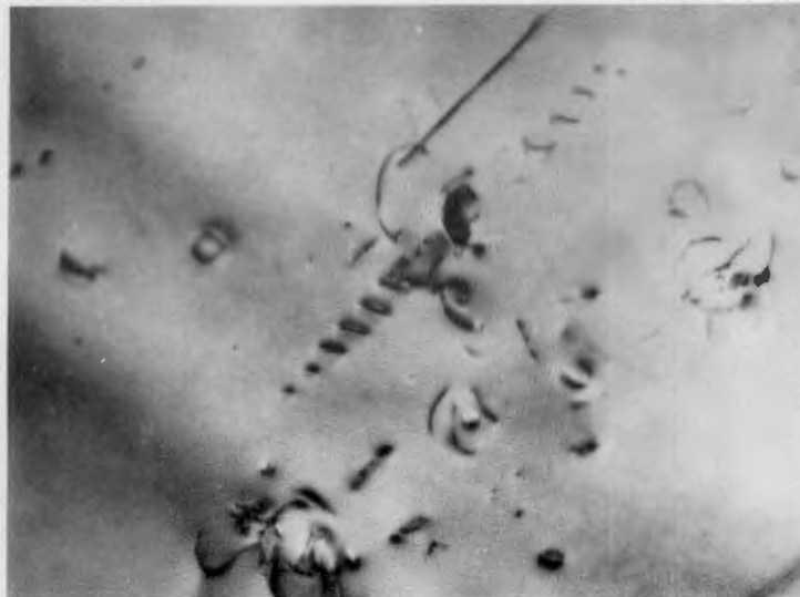
Fig. 4. Interstitial loops formed during carbide precipitation in 80 pct,Cr- Fe at 600°C.
