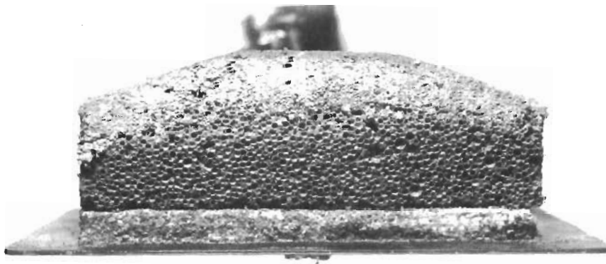
FIGURE 128 - 4000°F TEST SPECIMEN - 1.5 INCH RADIUS LEADING EDGE-BLOCK DESIGN (THERMAL TEST)
