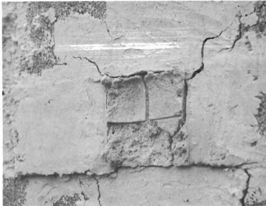
FIGURE 244 LOW DENSITY CHEMICALLY BONDED THO 2 (MAC LT-1) AFTER THERMAL TEST AT 4700°F
