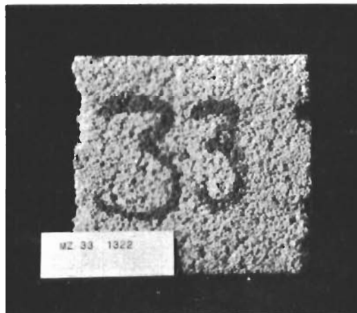
FIGURE 47 - ZIRCONIA BODY MZ33, THERMAL SHOCK TESTED - RATING 5.
