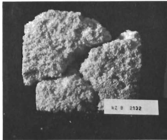
FIGURE 45 - ZIRCONIA BODY MZ8, THERMAL SHOCK TESTED - RATING 1.
