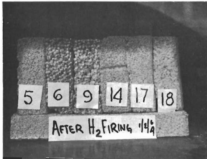
FIGURE 49 - LOW DENSITY ZIRCONIA BODIES FIRED IN HYDROGEN
