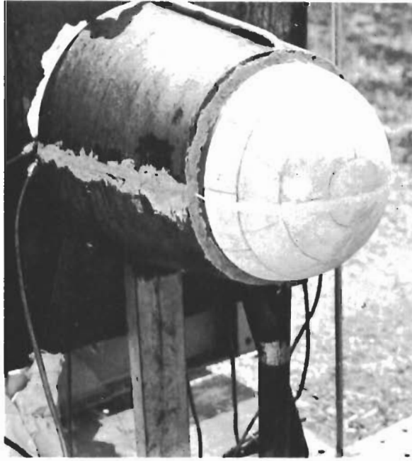
FIGURE 245 - 6.0 INCH RADIUS NOSE CAP READY FOR THERMAL TEST
