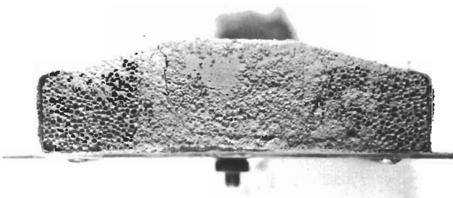
FIGURE 122 - 4000°F TEST SPECIMEN - 1.5 INCH RADIUS LEADING EDGE - HIGH DENSITY KEY BLOCK DESIGN ( THERMAL TEST )
