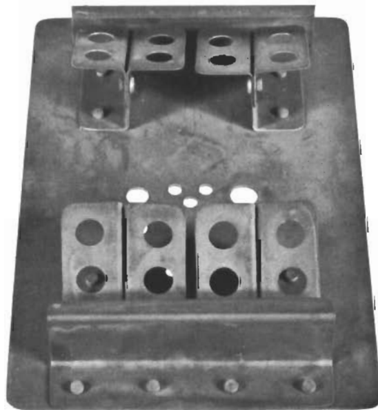
FIGURE 132 - METAL SUBASSEMBLY - 4000°F TEST SPECIMEN REINFORCED CHEMICALLY BONDED DESIGN
