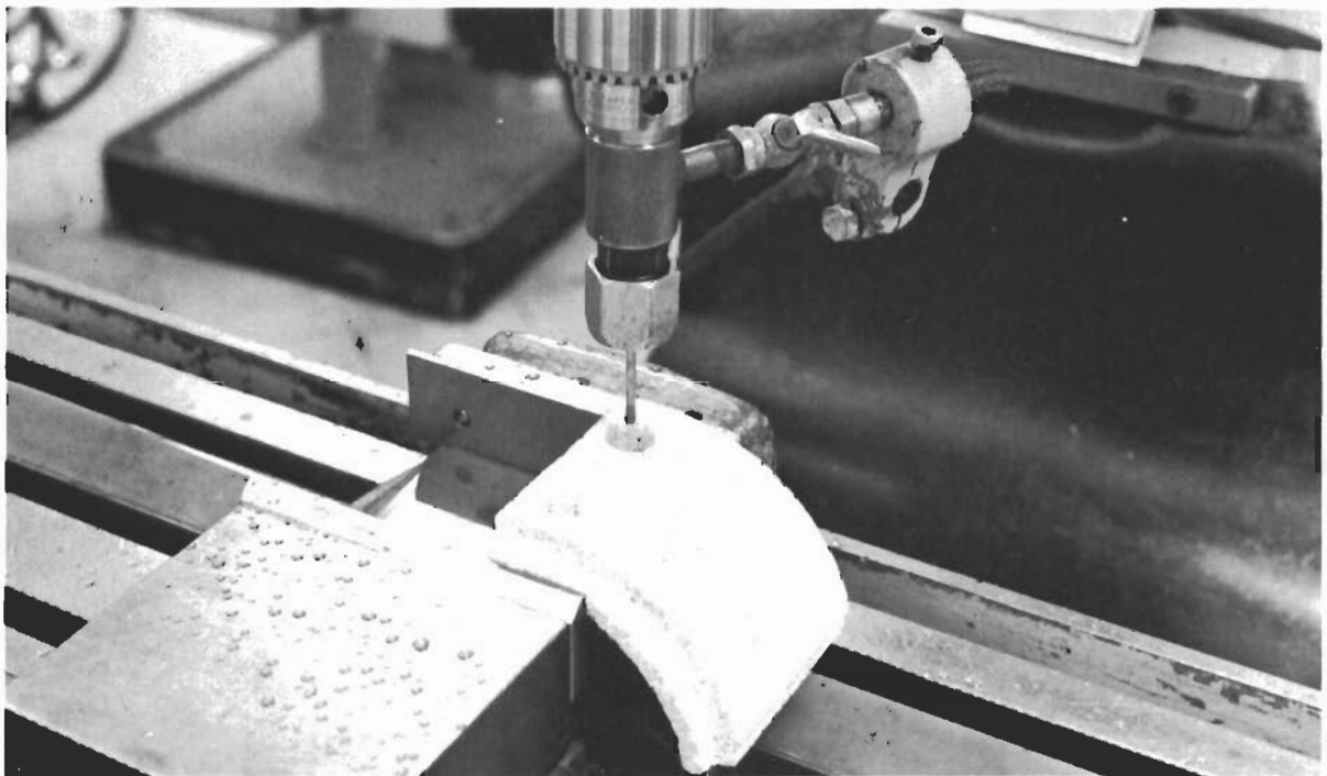
FIGURE 163 - DRILLING LOW DENSITY Al_2O_3 WITH A DIAMOND CORE DRILL
