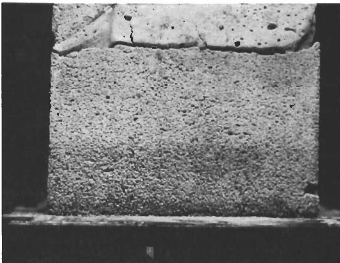
FIGURE 148 - 5000°F TEST SPECIMEN - NOSE CAP - TUBE REINFORCED CASTABLE DESIGN, REVISION A (THERMAL TEST)
