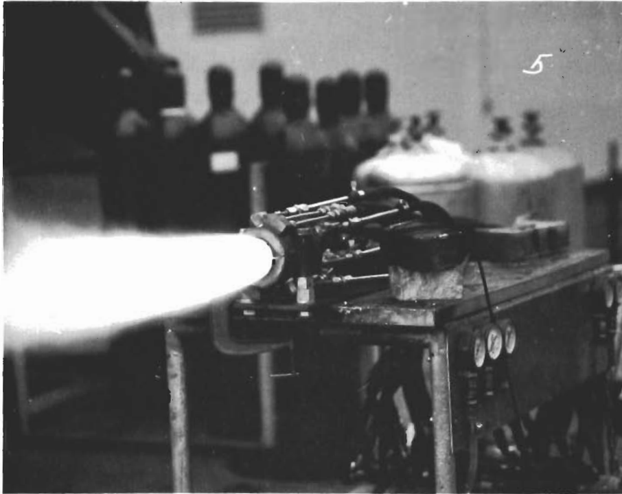
FIGURE 236 - TEST FIRING OF 2¼ INCH DIAMETER MAPP-OX BURNER
