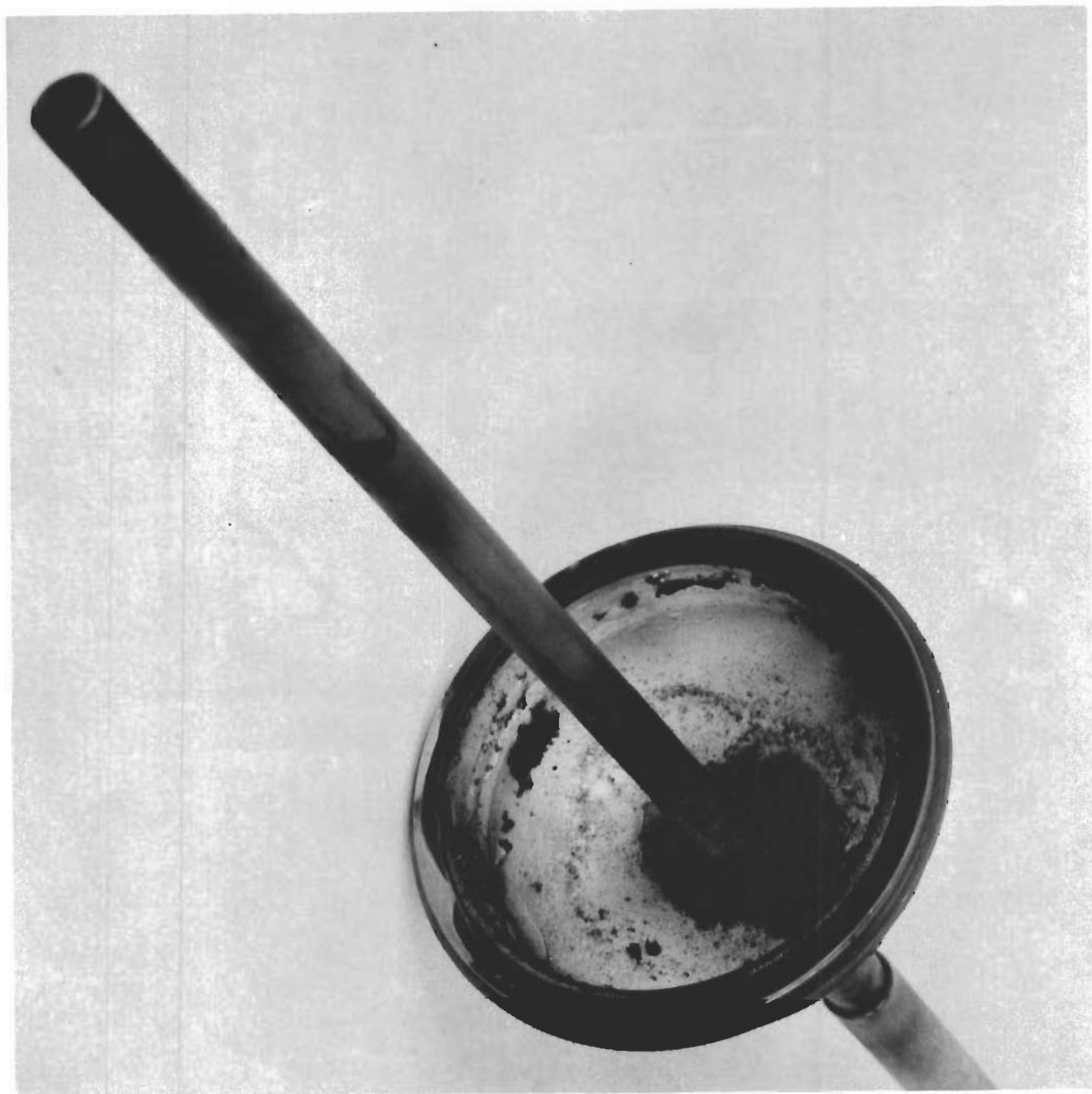
FIGURE 29. PHOTOGRAPH OF REACTOR-CAP AND INSIDE HEATER ASSEMBLY AFTER TEST
