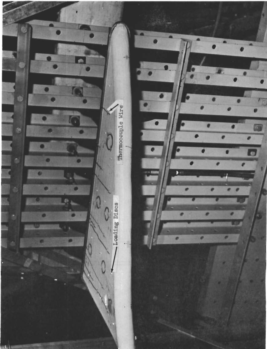
Figure 2 - Model One in Test Jig Showing Location of Load Deflection Points on Upper Surface
